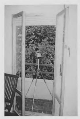
Figure A4.5: Outdoor noise measurements at each apartment.
