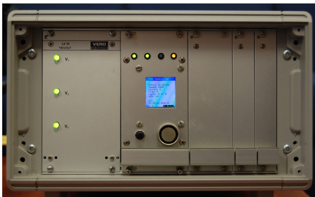
Figure 3.14 – Interface unit for controlling carriage motor and monitoring of sensors on the custom multi-material MSL system
