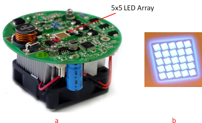
Figure 3.7 – A photograph of (a) an Enfis Uno Air Light engine [8] and (b) the observed array pattern when focused and projected onto a surface
