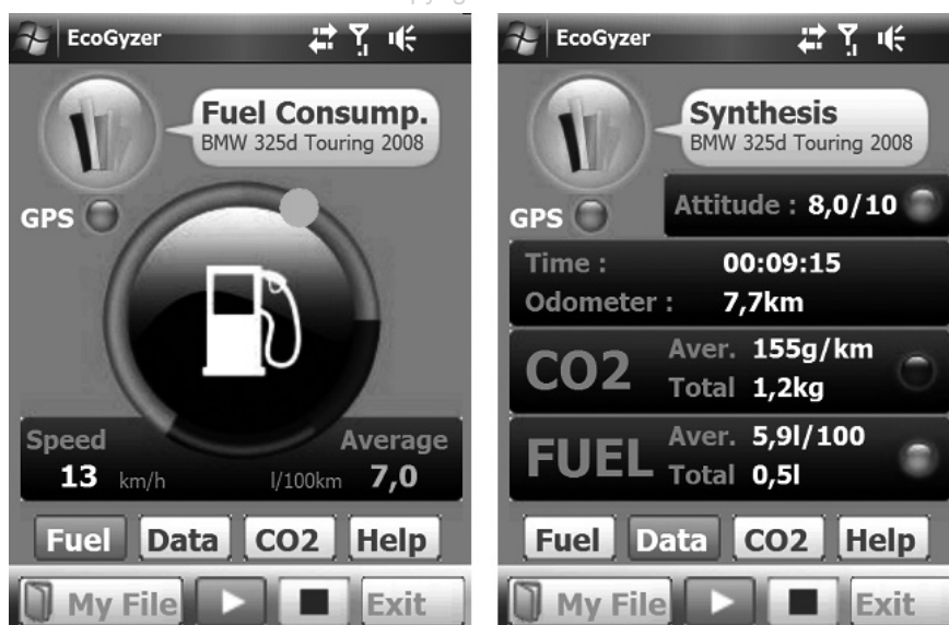
Figure 31.1 Main display of the EcoGyzer smartphone application seen during driving (left) and post trip summary (right)
