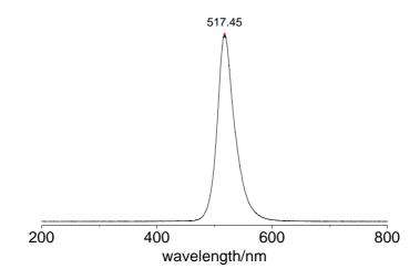
**Figure A.5** Output spectrum of High-Power 38 LED bulb/GU10 Green LEDs.
