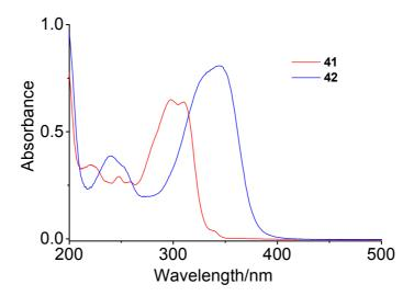
**Figure 6.5** UV-Vis pectra of MOPEP (**41**) and *cis*-[PtCl<sub>2</sub>(MOPEP)<sub>2</sub>] (**42**) in MeCN at 298 K. For compound **41**  $ε_{297nm} = 32445 \text{ M}^{-1} \text{ cm}^{-1}$ , **42**  $ε_{344nm} = 40420 \text{ M}^{-1} \text{ cm}^{-1}$ .
