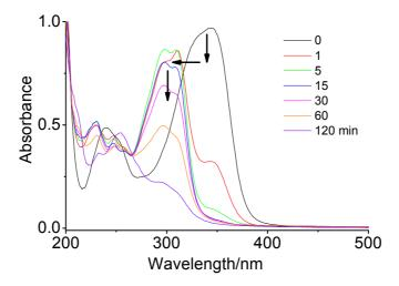
**Figure 6.6** Photoactivation of *cis*-[PtCl<sub>2</sub>(MOPEP)<sub>2</sub>] (**42**) upon irradiation with UVA ( $\lambda_{max} = 365 \text{ nm}, 3.5 \text{ mW/cm}^2$ , irradiation time 0, 1, 5, 15, 30, 60, 120 min) in MeCN at 298 K.
