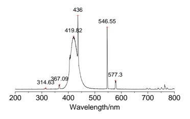
Figure A.3 Output spectrum of Luzchem LZC-420 lamps.
