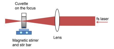
Figure 6.2 Instrument setup for TPA experiments.
