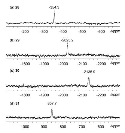
**Figure 5.5** <sup>195</sup>Pt NMR (129.4 MHz, 298 K) spectra of complexes (**a**) *trans*-[PtCl<sub>4</sub>(NH<sub>3</sub>)(4-NO<sub>2</sub>-Py)] (**28**); (**b**) *trans*-[PtCl<sub>2</sub>(NH<sub>3</sub>)(4-NO<sub>2</sub>-Py)] (**29**); (**c**) *trans*-[Pt(N<sub>3</sub>)<sub>2</sub>(NH<sub>3</sub>)(4-NO<sub>2</sub>-Py)] (**30**); (**d**) *trans*, *trans*, *trans*-[Pt(N<sub>3</sub>)<sub>2</sub>(OH)<sub>2</sub>(NH<sub>3</sub>)(4-NO<sub>2</sub>-Py)] (**31**).
