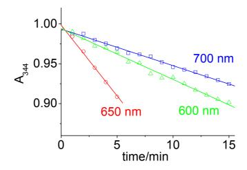
**Figure 6.11** Time-dependent decrease of absorbance at 344 nm for complex **42** by two-photon absorption. Power of the laser at these wavelengths: 600 nm, 16 μJ/pulse; 650 nm, 21 μJ/pulse; 700 nm, 21 μJ/pulse.
