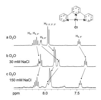
**Figure 5.18** <sup>1</sup>H-NMR of [Pt(Cl)(tpy)]Cl (**33**) (10 mM) in (**a**) D<sub>2</sub>O, (**b**) 30 mM NaCl in D<sub>2</sub>O, (**c**) 150 mM NaCl in D<sub>2</sub>O.
