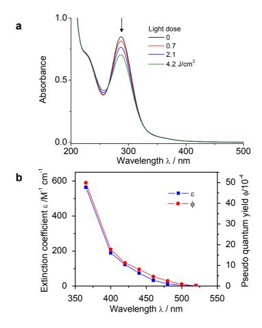
**Figure 5.6** (a) UV-Vis spectra for **31** in H<sub>2</sub>O upon irradiation at 365 nm. (b) Pseudo quantum yield  $\Phi$  (red, circles) of action spectrum (wavelength-dependent photodecomposition) for **31**, in comparison with extinction coefficient  $\varepsilon$  (blue, squares). The data points are the average of two experiments.
