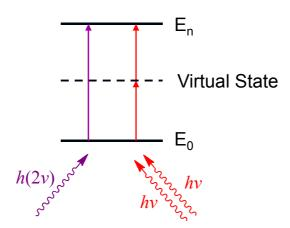
**Figure 6.1** Energy level diagram showing that the absorption of two photons from the red region (700 nm) can excite an atom of molecule to the same state as one photon from the violet region (350 nm).
