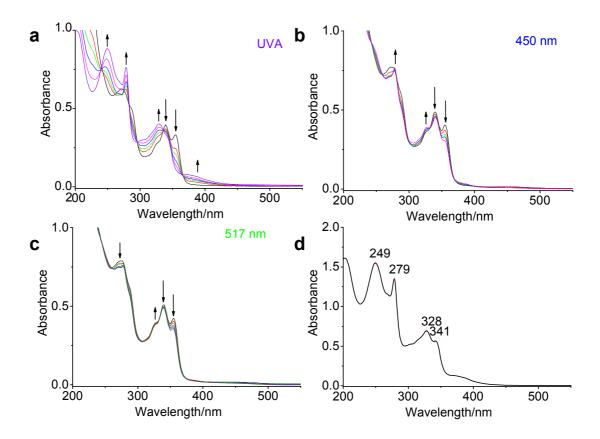
**Figure 5.15** UV-Vis spectra recorded for *trans*-[Pt(N<sub>3</sub>)(OH)<sub>2</sub>(Tpy)]Cl (**36**) in H<sub>2</sub>O upon irradiation with (**a**) UVA (4.55 mW/cm<sup>2</sup>, irradiation time 0, 0.5, 1, 2, 5, 30 min), (**b**) at 450 nm (50 mW/cm<sup>2</sup>, irradiation time 0, 5, 15, 30, 60 min) and (**c**) 517 nm (50 mW/cm<sup>2</sup>, irradiation time 0, 5, 15, 30, 60, 120 min) at 298 K. (**d**) UV-Vis spectrum of [PtCl(Tpy)]Cl (**33**) in H<sub>2</sub>O.
