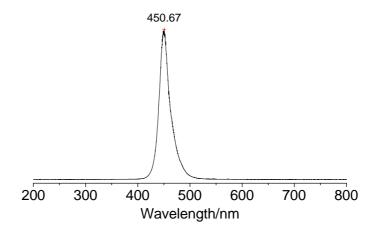
**Figure A.4** Output spectrum of ACULED® VHL<sup>TM</sup> 450 nm LEDs.
