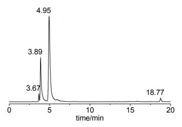
**Figure 5.13** Typical HPLC chromatogram for **36** raw product. Semi-preparative HPLC was used to purify the product. The peak at retention time of 4.95 min was collected. HPLC conditions: HP1100 series. Column: Agilent ZORBAX Eclipse XDB-C18,  $9.4 \times 250$  mm, 5  $\mu$ m. Flow rate, 2 ml/min. Detection wavelength: 254 nm. Mobile phase A, H<sub>2</sub>O with 0.1% TFA; B, MeOH with 0.1% TFA. The gradient used is the same as shown in **Figure 5.11**.
