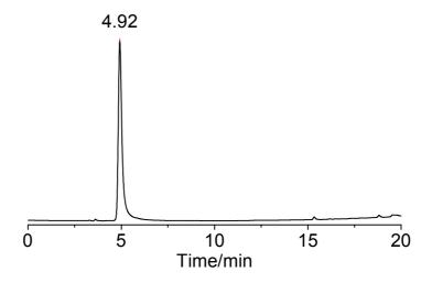
**Figure 5.14** Product of complex **36** after HPLC purification. The purity was >95%. The same HPLC method was used as that in **Figure 5.13**.
