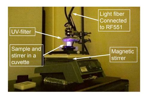
**Figure 5.1** Instrument setup for the action spectrum.
