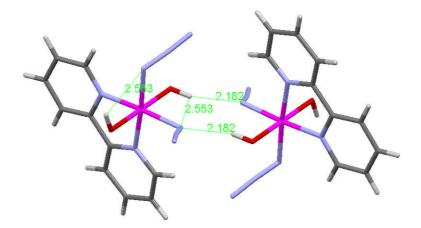
**Figure 5.10** Intra- and inter-molecular H-bonds network formed by azido and hydroxido ligands in the structure of complex **32** which determines the orientation of the azido ligands.
