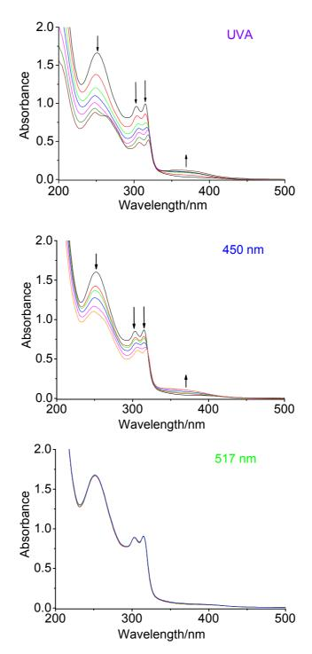
**Figure 5.12** Photoactivation of complex *cis, trans*-[Pt(N<sub>3</sub>)<sub>2</sub>(OH)<sub>2</sub>(Bpy)] (**32**) in H<sub>2</sub>O upon irradiation with UVA (0, 1, 2, 3, 5, 15, 60 min), 450 nm (0, 10, 15, 30, 60, 120 min ) and 517 nm (0, 5, 30, 60 min) (298 K).
