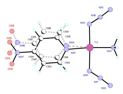
**Figure 5.4** The disorder of the 4-nitopyridine ligand in one of the molecules (Pt3 complex) in the solid state structure of *trans*-[Pt(N<sub>3</sub>)<sub>2</sub>(NH<sub>3</sub>)(4-NO<sub>2</sub>-Py)] **30** showing the two orientations of the 4-nitropyridine ligand about the 2-fold axis. There is a 50:50 occupancy of the two orientations, one drawn with solid lines and one with dashed lines.
