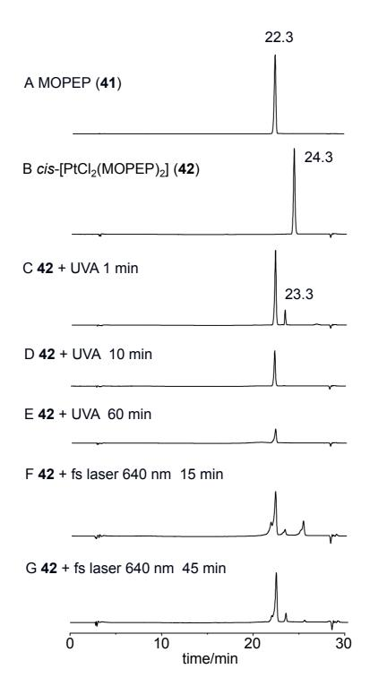
**Figure 6.10** HPLC analysis of **(A)** MOPEP **(41)** (RT = 22.3 min); **(B)** *cis*-[PtCl<sub>2</sub>(MOPEP)<sub>2</sub>] **(42)** (RT = 24.3 min) and the photolysis of **42** in MeCN upon irradiation with UVA  $(3.5 \text{ mW/cm}^2)$  for **(C)** 1 min, **(D)** 10 min, **(E)** 60 min; and upon irradiation with a focused 640 nm fs laser light **(F)** 15 min, **(G)** 45 min. Detection wavelength: 315 nm.
