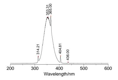
Figure A.1 Output spectrum of Hitachi UVA lamps.
