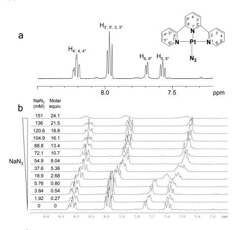
Figure 5.19 <sup>1</sup>H-NMR analysis for  $[Pt(Tpy)(N_3)](N_3)$  (34). (a)  $[Pt(Tpy)(N_3)](N_3)$  (7.16 mM) in D<sub>2</sub>O. (b)  $[Pt(Tpy)(N_3)]N_3 + NaN_3$  (0 – 151 mM) in D<sub>2</sub>O. The concentration of NaN<sub>3</sub> over 151 mM lead to the precipitation of 34.
