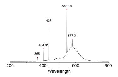
Figure A.2 Output spectrum of Hitachi visible lamp.
