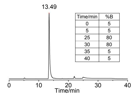
**Figure 5.11** HPLC chromatogram for complex *cis, trans*-[Pt(N<sub>3</sub>)<sub>2</sub>(OH)<sub>2</sub>(Bpy)] (**32**) based on peak areas. Purity is > 95%. HPLC conditions: HP1100 series. Column: Polymer Laboratories, PLRP-S, 250×4.6 mm, 100 Å, 5  $\mu$ m. Flow rate, 1.00 ml/min. Wavelength: 254 nm. Mobile phases A, H<sub>2</sub>O, 0.1% TFA; B, MeOH, 0.1% TFA. Insertion is the gradient of mobile phases used.
