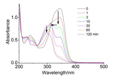
**Figure 6.7** Photoactivation of *cis*-[PtCl<sub>2</sub>(MOPEP)<sub>2</sub>] (**42**) with white light ( $\lambda \sim 400 - 700 \text{ nm}$ , 12 mW/cm<sup>2</sup>, irradiation time 0, 1, 3, 10, 30, 60, 120 min) in MeCN at 298 K.
