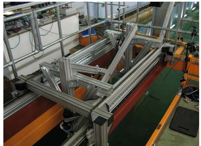
Fig. 2. Photo of the turbine as installed, with the main and auxiliary carriages visible.
