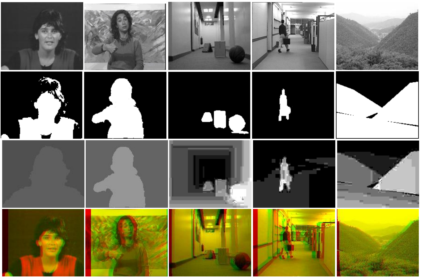
Fig. 7: Results extracted from five test sequences including “Miss America”, “silence”, “Aisle1”, “Hall monitor”, and “Mountain” (from left to right). From top to bottom, four rows respectively correspond to original image, segmented results, estimated depth maps, and synthesized stereo image.
