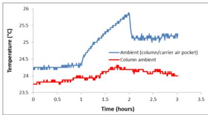
Figure 3: Ambient temperature inside column/carrier air pocket
