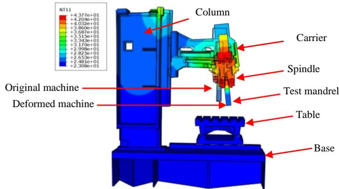
Figure 8: Simulated visual representation of deformation of the machine due to internal heating
