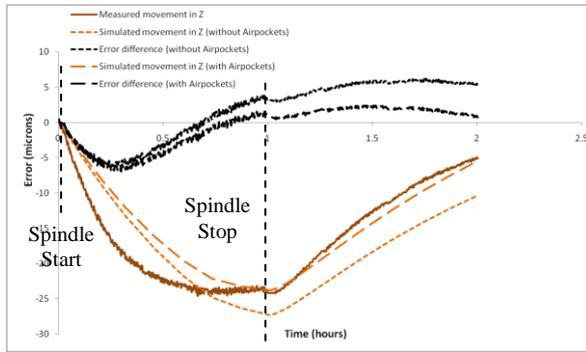
Figure 7: Z-Displacement profiles correlation (8000rpm)
