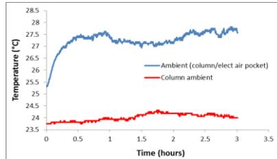
Figure 5: Ambient temperature inside column/elect air pocket
