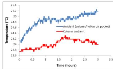
Figure 4: Ambient temperature inside column/hollow air pocket
