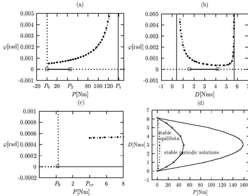
Figure 3.1: (a), (b) Bifurcation diagrams, the bifurcation parameter is  $P$  and  $D$ , respectively (c) The bifurcation diagram near the point where the computation is interrupted (d) The stability chart with the bifurcation curves
