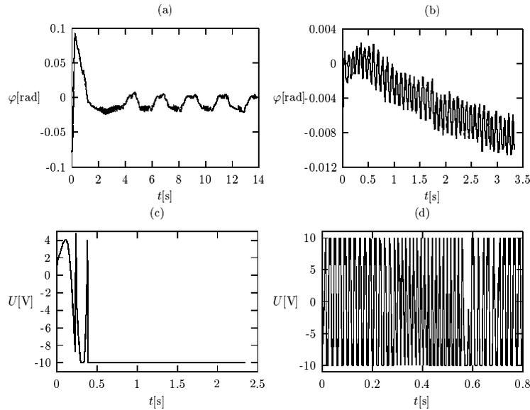
Figure 5.2: Time evolutions for different controllers (a)  $P = 100$  [Nm],  $D = 6$  [Nms] (b)  $P = 700$  [Nm],  $D = 6$  [Nms] (c)  $P = 100$  [Nm],  $D = 2$  [Nms] (d)  $P = 700$  [Nm],  $D = 23$  [Nms]
