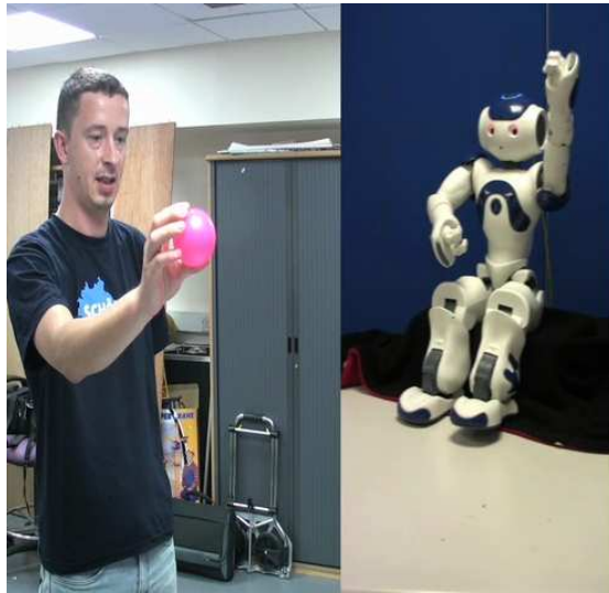
Fig. 1: Experimental setup. The human partner is in front of the robot, moving a pink ball between the four different positions in the visual field. The robot learns the proper response to mirror the actions of the human partner.
