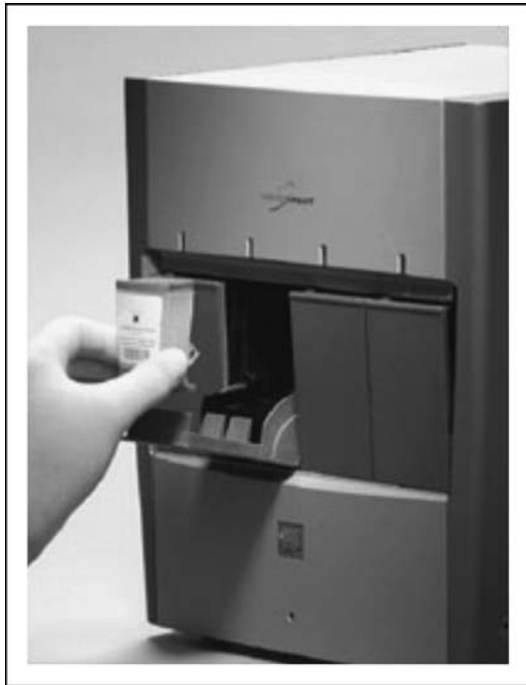
Figure 3 Cepheid GeneXpert IV and Xpert MTB/RIF test cartridge
