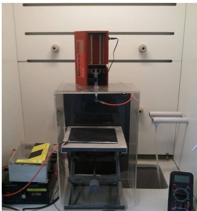
Figure 18: Electrospinning apparatus set up within a fume cupboard.
