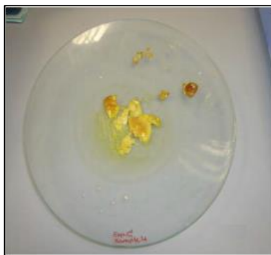
Figure 17: Wet biomass left to dry on a pre-weighed watch glass.
