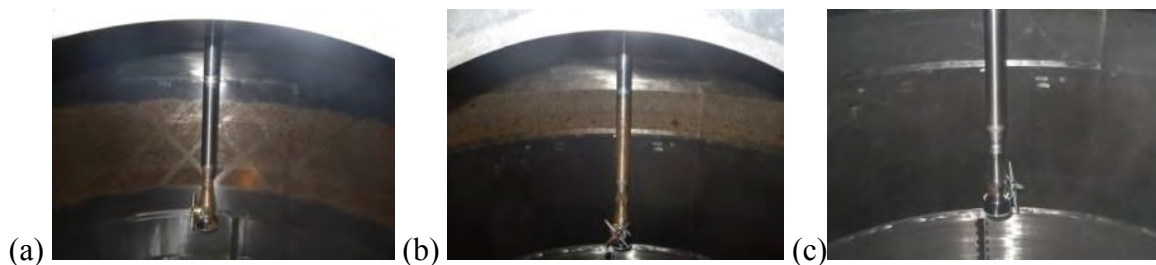
Figure 3.25: Phases of CIP (a) After 1 minute of pre-rinse, (b) after 8 minutes of pre-rinse (c) after the chemical phase and final rinse.
