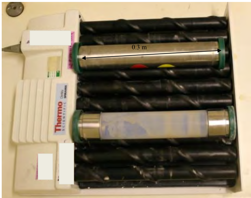
Figure 3.36: Section of 0.3 m pipe (stainless steel and plastic, 2" OD) on the roller mixer placed in an incubator at 30°C.
