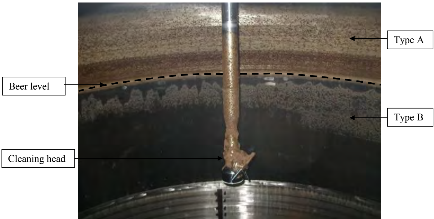
Figure 1.2: View into the top of a fermenter (through man way door) after fermentation prior to cleaning.
