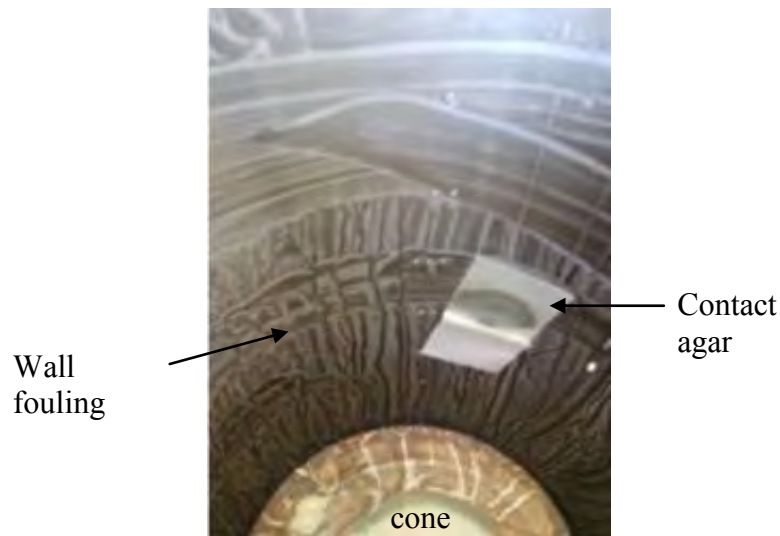
Figure 2.4: 80 l stainless steel tank (0.8 m by 0.4 mm) with residual yeast fouling attached to the wall and the cone. The wall was also sampled by contact agar (from Salo et al., 2008).
