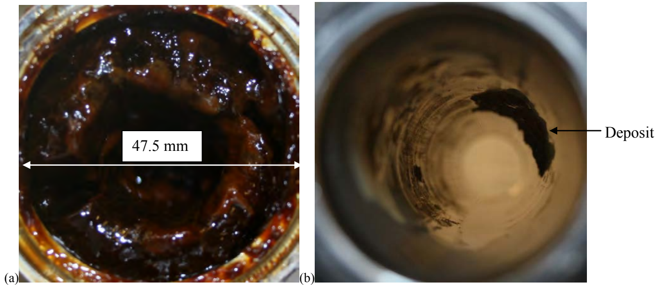
Figure 6.4: Cooked caramel deposit in 0.5 m section of pipe (on left) and after a pre-rinse at 1.5 \text{ m s}^{-1} at 50^\circ\text{C} (on right).
