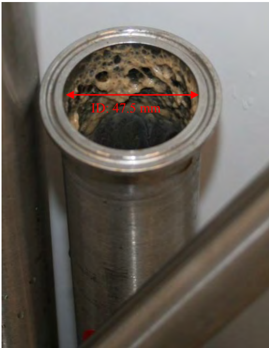
Figure 3.35: Fouling layers obtained from vertical pipe fermentation with head space of 25 %.
