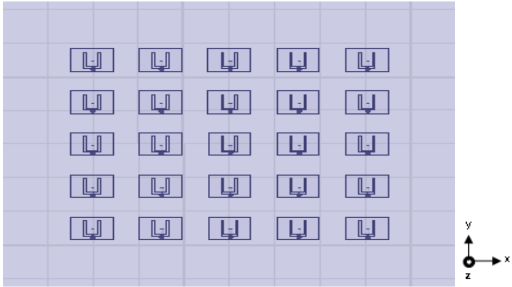
Fig. 4.6. 5x5 U-slot array with E-plane patch orientation [64] (© 2014 IEEE)
