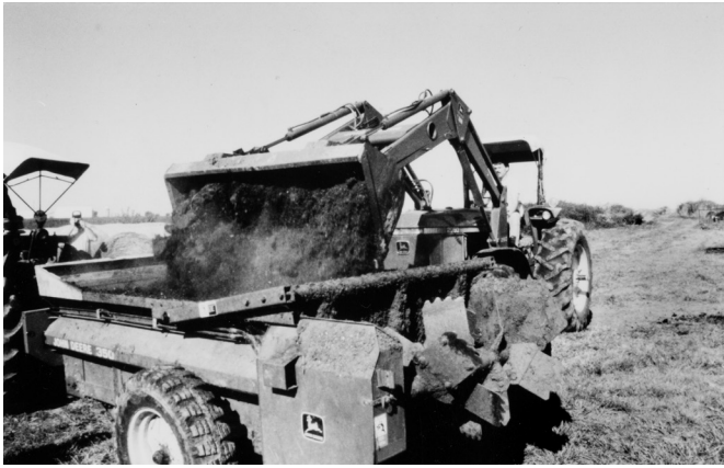
Figure 7. A front-end loader and beater-type spreader work well for loading and field-spreading compost.
