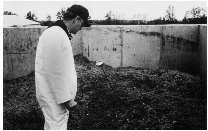
Figure 8. Temperature is the best indicator of the conditions of the composting material.
