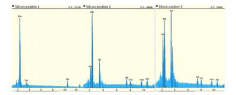
Figure 92: EDX analysis on pad 1 (silicon). Position numbers reflect the one in figure 89. The normalized results are: Pb 76 wt%, Au 6 wt.%, Sn 18 wt.% in the 10x10  $\mu m^2$  area and, Pb 26 wt.%, Au 28 wt.%, Sn 46 wt.% in the 3x3  $\mu m^2$  area.
