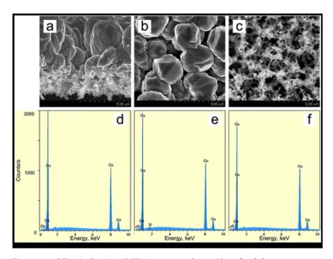
Figure 64: SEM (a, b, c) and EDX point analyses (d, e, f) of the porous copper membrane. The porous copper membrane was formed by displacement deposition of copper on 0.3  $\Omega cm$  p-type silicon for 7,200 s from the solution containing IPA (improved wettability); porous copper membrane was analyzed in cross section (a, d), top (b, e), and bottom (c, f).
