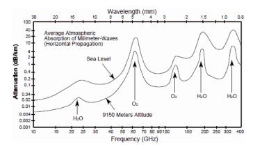
Figure 122: The average atmospheric absorption in the 10 to 400 GHz frequency range (without fog or rain contributions) at sea level and 9150m of altitude.
