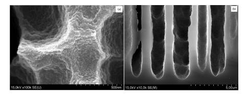
Figure 43: Roughness of the surface of macro-PS layer.
