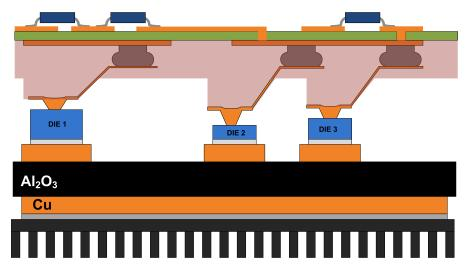
Figure 120: An improved IHPM with the same connectivity exploiting the top board to replace two long wires contacting the substrate.
