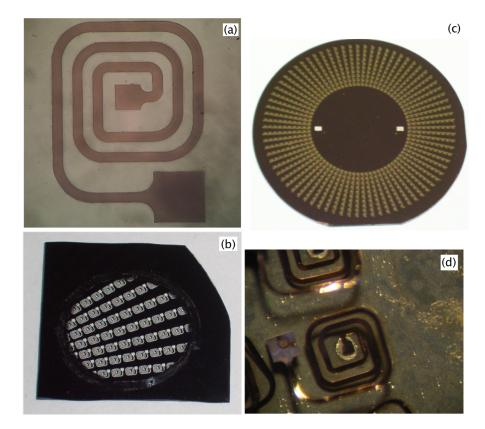
Figure 121: First prototypes of the u-helix antenna design: (a) planar structure of a single antenna; (b) quarter of a silicon wafer for testing processes for the realization of an array of u-helices; (c) full 4 inches wafer with a circular array of more than 300 antennas; (d) u-helix antenna after the pulling process, stabilized in a transparent polymer.
