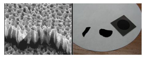
Figure 108: Detached macroporous membrane. The SEM image shows the membrane morphology in a region corresponding to a crack. The photo shows the an example of a separate membrane (broken in two pieces) and a membrane is still on a silicon wafer. Sample has been realized in HF:DMSO (10:46) at 10  $mA/cm^2$  for 30 min, *HF* 45% at 40  $mA/cm^2$  for 10 min, and HF:DMSO (10:46) for 1 min.
