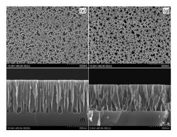
Figure 41: 80% porosity meso-PS layers on n+ type: (100)-oriented silicon wafer (left) and (111)-oriented silicon wafer (right) with resistivity of 0.01  $\Omega$ cm.
