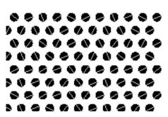
Figure 148: Feret's diameters extracted for the holes in the test image. The image represents only a part of the original image to make visible the Feret's diameters.
