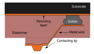
Figure 113: The compliant contact realized with CRML technology.
