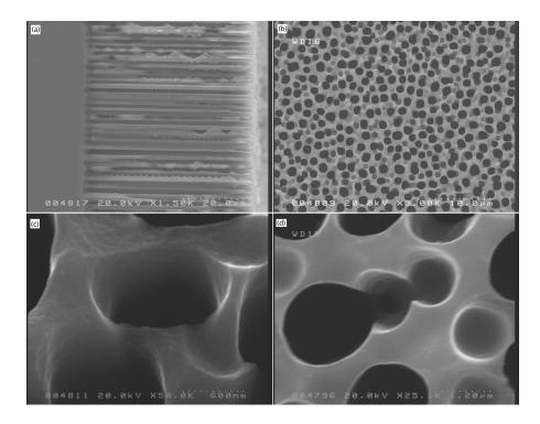
Figure 42: SEM images of macroporous silicon layer obtained on 10-20  $\Omega cm$ , p-type, (100)-orientation, with HF:DMSO (10:46) at 10  $mA/cm^2$  for 60 minutes, at RT. (a) Cross section of the layer (thickness of 55  $\mu m$ ); (b) top-view of the layer; (c) Magnification of the "entrance" of a pore; (d) magnification of a fully developed pore and two associated interpores.
