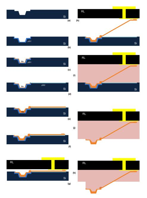
Figure 86: Main technological step for the realization of the electrical contact: (a) etching of pyramid pattern, (b) realization of the highadhesion porous silicon layer, (c) deposition of contact metal, (d) realization of the low-adhesion porous silicon layer, (e) deposition of wire meal, (f) deposition of the "pulling-pad" metal, (g) alignment with the RL substrate, (h) pulling process, (i) polymer filling, (j) silicon wafer separation, (k) polymer etch for contact definition.
