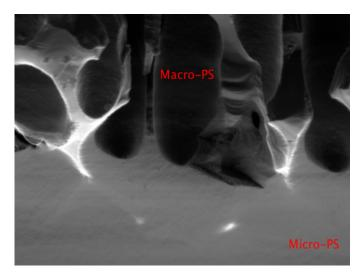
Figure 104: SEM image of the interface between macroporous layer (top) and microporous layer (bottom). The interface is continuous with microporous layer surrounding the bottom of the macropores.
