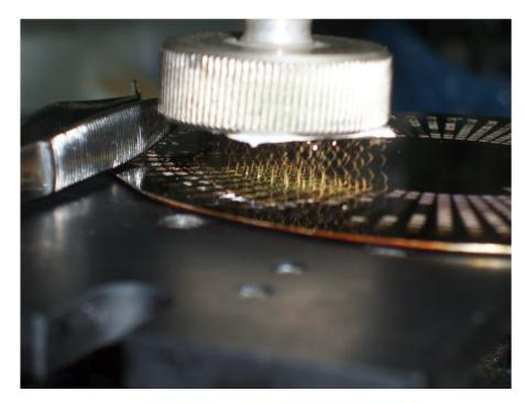
Figure 137: On-chip integration of u-helix test. Part of the circular array (bottom) has been bonded to a dummy die consisting of pads only (top). Pulling is done on a manual setup. The antennas have been extended beyond the optimum height photographing purposes.
