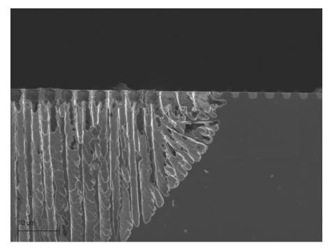
Figure 50: Ordered macropores obtained on p-type (100)-orientation silicon wafer with a resistivity of 10-20  $\Omega cm$ . The macro-PS layer has been obtained in HF:DMSO (10:46) at a current density of 10  $mA/cm^2$  for 45 minutes. Pre-pitting of the substrate (2  $\mu m$  opening, 4  $\mu m$  pitch, 1.5  $\mu m$  depth) has been done with RIE.
