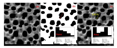
Figure 3: Example of image analysis of macroporous silicon done with ImageJ. The original SEM image on the left (a) is thresholded and analyzed with ImageJ *particles analysis tool* (b), and the distribution of dimensional parameters of the pores are extracted (c and insets).
