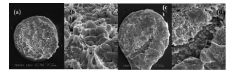
Figure 90: SEM images of pad 1; ceramic side (a), magnification of pad1 to reveal intermetallic compounds (b); silicon side (c) and magnification of fracture on silicon side (d).
