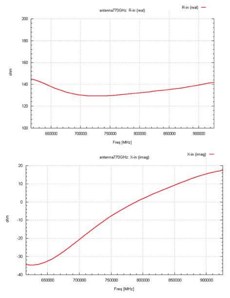
Figure 135: Real and imaginary part of the input impedance of the 1 THz u-helix antenna simulated with NEC2.
