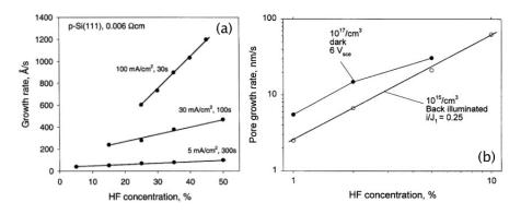
Figure 20: Growth rate of pores as a function of HF concentration: (a) p-type silicon [25], (b) n-type silicon [26].
