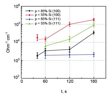
Figure 63: Conductivity of copper films deposited on PS using the immersion displacement deposition.
