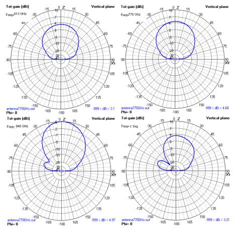
Figure 134: Radiation pattern of the 1THz u-helix antenna simulated with NEC2.
