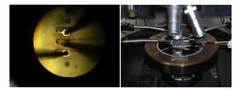
Figure 115: The measurement setup for the contact resistance. The panel on the left shows the three probes contacting the tips. The panel on the right shows the set-up.
