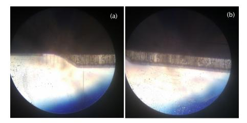
Figure 102: Edge (a) and center (b) image at the optical microscope (50x objective, each mark is 7.4  $\mu$ m) of a sample realized with: HF:DMSO (10:46) with 10  $mA/cm^2$  for 30 min, and HF 45% with 40  $mA/cm^2$  for 20 min, at RT. Silicon was masked with SU-8 photoresist, under-etching due to peeling if the photoresist at the edge is visible.
