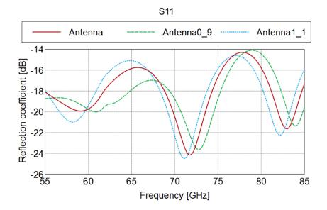
Figure 132: Return loss (S11) for the 55GHz u-helix antenna (at nominal height and for  $\pm 10\%$  variations.
