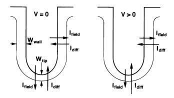
Figure 38: (a, left) Equilibrium (V=o) field currents and diffusion currents across the space-charge region for the macropore tip and wall region in p-type silicon. (b, right) Field currents and diffusion currents under forward bias (V>o). Note that due to geometric field enhancement around the pore tip the tip currents are always larger than the pore wall currents [16].
