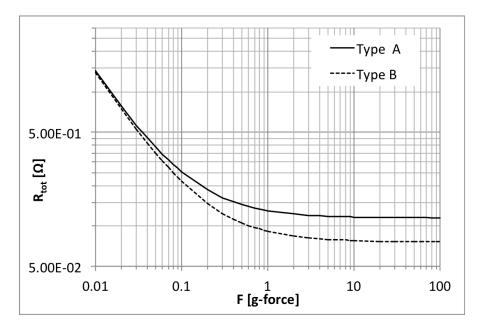
Figure 114: Total resistance of the single probe for both types of contact structures for contact forces between 0.01 and 100 grams-force on a log/log scale.
