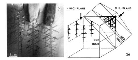
Figure 15: (a) Dendritic PS morphology formed on n-type (100) [23]; (b) Schematic illustration of the growth direction of dendritic PS in relation to the crystal orientation of the silicon sample [21].
