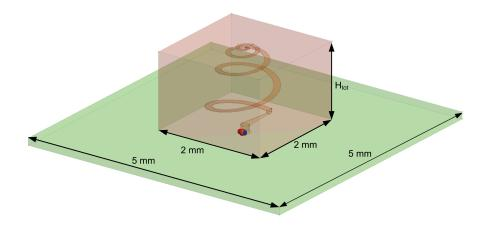
Figure 129: Model for the MoM simulator of the 55 GHz u-helix antenna. The antenna is embedded into a 2mm x 2mm x H<sub>tot</sub> dielectric cube made of silicone,  $\epsilon_r = 2.33$ ) and over a 0.127 mm dielectric substrate. Ground plane is at the bottom and the arm visible in the figure centrally feeds the antenna (through a via hole in the substrate).
