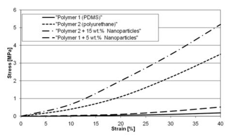
Figure 96: Stress strain diagram for different polymers.
