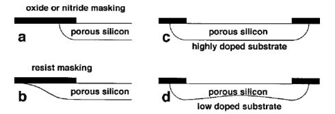
Figure 31: PS layer thickness inhomogeneities as a result of different kinds of masking layers and doping densities. (a) While under-etching is minimal for a silicon nitride mask, (b) a resist mask shows severe under-etching. (c) On substrates of low resistivity the etch profile is isotropic, (d) while the PS thickness increases towards the edges of the pattern for high substrate resistivities [17].
