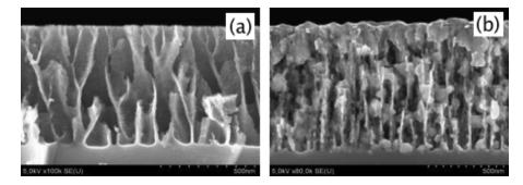
Figure 84: SEM cross section image of porous silicon as fabricated (a) and after metal deposition (b).
