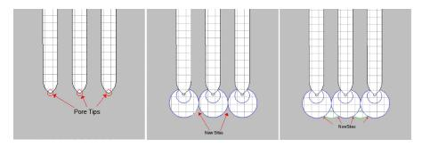
Figure 110: Growth model for microporous silicon layer below a macroporous layer: growth starts at pore tips (left), and proceed with a spherical front in all directions until two spherical front touches (center) forming a new sharp tip facing upward in correspondence of the contact point. A new nucleation site starts in correspondence of the contact point and the growth proceeds (right).
