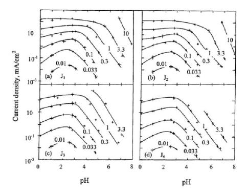
Figure 18: Plots of the characteristic current densities  $J_1$  (a),  $J_2$  (b),  $J_3$  (c), and  $J_4$  (d) as a function of pH, for different values of fluorine concentration (labeled on the curves in units of mol/liter).
