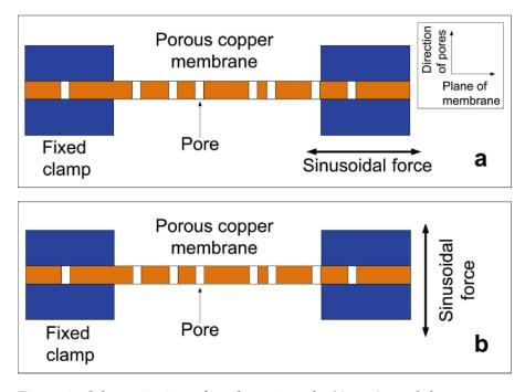
Figure 65: Schematic view of configurations for Young's modulus measurements: (a) Tensile configuration  $E_{\perp}$ , (b) cantilever configuration  $E_{\parallel}$ .
