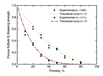
Figure 9: Relative (to bulk silicon) breaking strength of meso-PS layers (10  $\mu m$  thick) with porosities between 10% and 80% [20].
