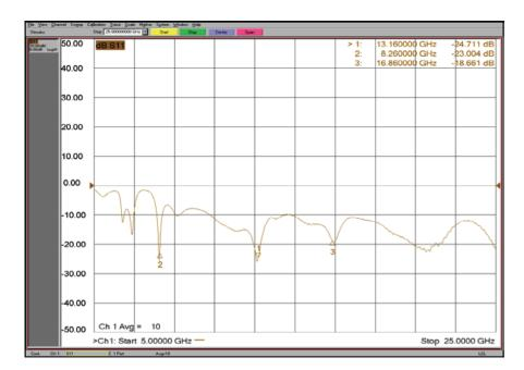
Figure 140: Measured S11 for the 10 GHz prototype.
