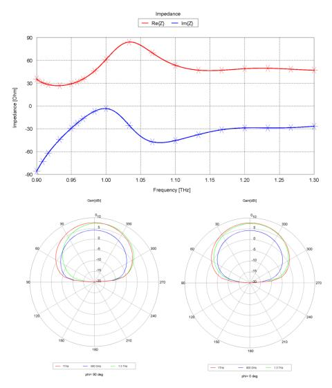
Figure 138: Simulated U-Helix antenna impedance (top) and radiation pattern (bottom) for two different  $\varphi$  angles (0 and 90°).
