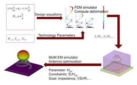
Figure 125: Design procedure for u-helix antennas is a combination of mechanical and electromagnetic simulations to optimize the final geometry.
