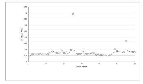
Figure 117: The resistance values measured for contactor A over 60 different pads.
