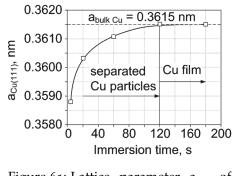
Figure 61: Lattice parameter  $a_{Cu}$  of Cu (111) vs immersion time.
