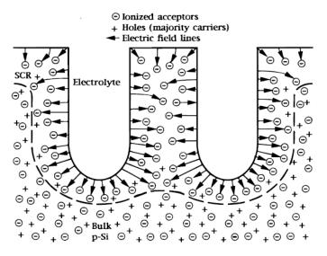
Figure 37: Sketch of the equilibrium charge distribution and the electric field around pores in a p-type semiconductor electrode.
