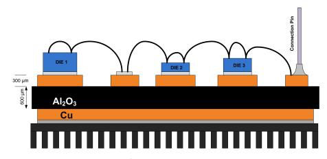
Figure 118: Representation of an Integrated Power module (IPM). Power devices (DIE1, DIE2 and DIE3), of different heights are soldered over a DBC substrate (300 um thick copper bonded on 600 µm alumina) and connected with thick (300 µm) aluminum bond wires. On the backside an heat sink is soldered for thermal dissipation. Connection pin brings control signal to an external control electronics.
