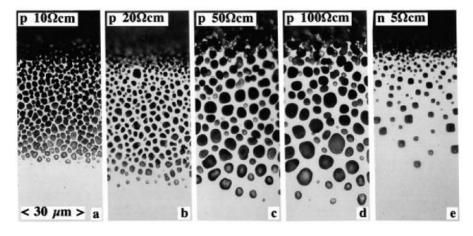
Figure 10: (a-d) Optical micrographs of p-type substrates of different doping densities polished under a small angle to the electrode surface, after anodization under identical conditions in the dark (10% aqueous HF, 3 mA cm<sup>-2</sup>, 90 min). (e) An n-type substrate anodized under similar conditions is shown for comparison (10% HF, 3 mA cm<sup>-2</sup>, 30 min) [17].
