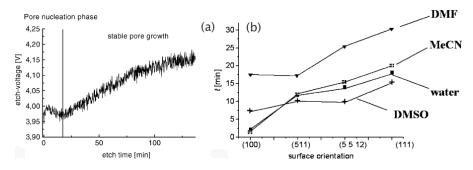
Figure 24: Nucleation time of macropores: (a) Development of the voltage over time for constant current and a DMF electrolyte. A nucleation phase and a stable growth phase can always be identified.(b) Nucleation time for various electrolytes and surface orientations [27].
