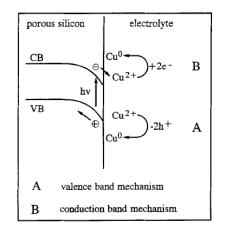
Figure 67: Reduction mechanism of copper on silicon electrodes [33].
