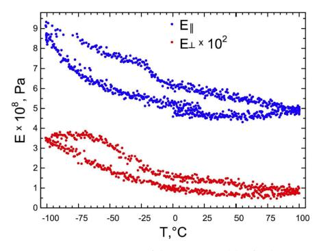
Figure 66: Temperature variation of the Young's modulus for the copper membrane. The modulus is computed in two directions: perpendicular and parallel to the porous structure.
