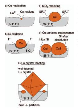
Figure 59: Phenomenological model of copperPS particles growth on PS skeleton.
