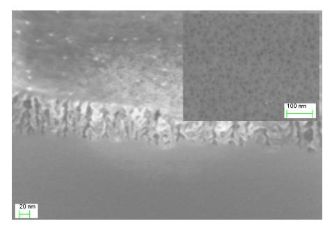
Figure 7: SEM image of the cross-section and the top-view (inset) of a meso-PS sample (from a p+ wafer) with a porosity of about 50%.
