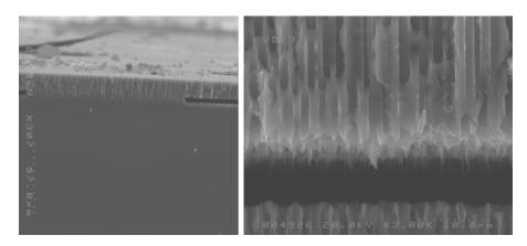
Figure 107: Cross-sections of a buried cavity surrounded by macro-PS on all sides. Sample has been realized in HF:DMSO (10:46) at 10  $mA/cm^2$  for 30 min, HF 45% at 40  $mA/cm^2$  for 20 min, and HF:DMSO (10:46) for 1 min at 10  $mA/cm^2$ , RT.
