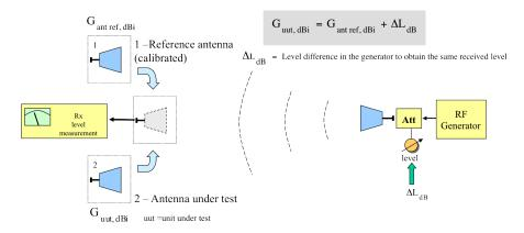
Figure 141: Antenna measurement methodology. A comparison measurement methodology has been employed to measure the gain of the u-helix antenna.
