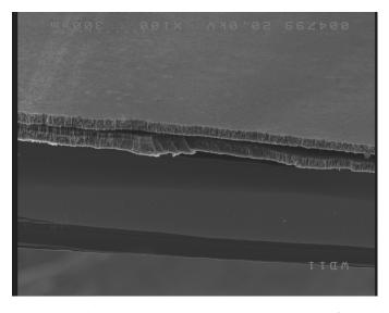
Figure 101: Multilayer macroporous structure detached from silicon.
