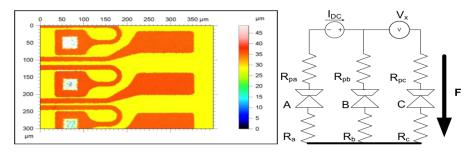
Figure 116: Profilometer images of three test pads (left) and three-points measurement technique (right).
