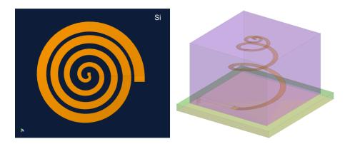
Figure 123: Top (left) and perspective view (right) of the actual design of the u-helix antenna. The perspective view shows the antenna conductor is embedded in a polymer and placed over a dielectric substrate and fed with a microstrip.
