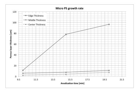
Figure 52: Micro-PS growth for HF 45 wt.% on p-type (100)-oriented 10-20  $\Omega cm$  silicon wafer, process rate. Data are sampled in three different points (see 3.3.3 for a description of the sampling strategy).
