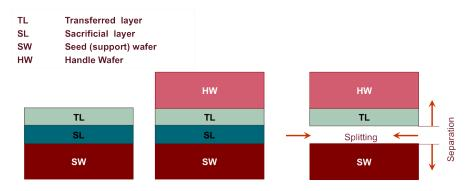
Figure 80: Layer transfer technology definitions and steps.
