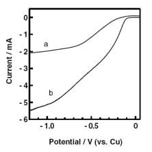
Figure 68: Current-potential curves of macroporous silicon measured in 0.1 M CuSO<sub>4</sub>: (a) in the dark, and (b) under front-side illumination. The scan rate was 10 mV/s [33].
