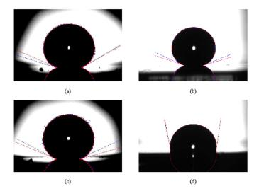
Figure 76: Contact angles on selected silanized samples: (a) sample 1, (b) sample 2, (c) sample 3 as defined in table 6, corresponding to processes A-C, respectively in table 5; (d) silanized flat silicon wafer.
