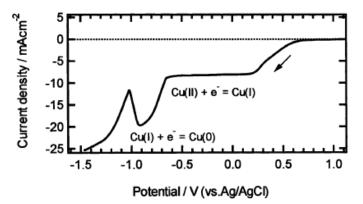
Figure 55: Current density-potential curve of platinum rotating disk electrode in 0.01 M  $(CF_3SO_3)_2$ Cu MeCN solution containing 0.1 M tetra-*n*-butylammonium perchlorate as supporting electrolyte. The rotation rate and scan rate were 2000 rpm and 10  $mVs^{-1}$ , respectively [32].
