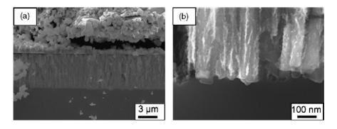
Figure 71: Cross-sectional views of the mesoporous silicon with 4  $\mu m$  depth after the copper electrodeposition at -5A for 2 h (sample areao.79*cm*<sup>2</sup>): (a) low magnification image, and (b) high magnification image [35].
