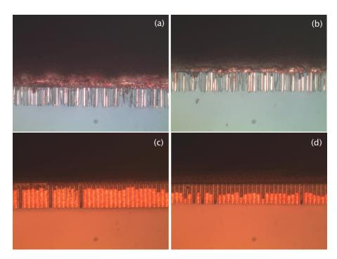
Figure 75: Examples of macroporous structures filled with copper. Both random macropore layers (a,b) and ordered have (c,d), have been filled. The macropores were grown into 10-20  $\Omega cm$  (100)-oriented, p-type wafer.
