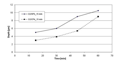
Figure 94: Etching rate of polyurethane in RIE with  $SF_6/O_2$  and  $SF_6/CF_4$  gases.
