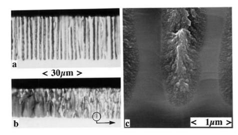
Figure 11: (a,b) Cross-sectional optical micrographs of macroporous silicon formed by anodization of (100) p-type 20  $\Omega cm$  silicon electrodes in (a) 2 M HF in MeCN (3  $mA cm^{-2}$ , 90 min, RT) and in (b) 30% aqueous HF (40  $mA cm^{-2}$ , 7.5 min, RT). (c) A SEM micrograph of the macropores in (b) reveals that most of the pore volume is filled with microporous silicon [17].
