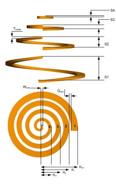
Figure 124: The u-Helix antenna with dimensional parameters in lateral and top views. In the top half of the antenna the four loops (each loop isolated for clarity) are shown, with the definition of spacings (S1 to S4). In the bottom half, the top view of the spiral is shown, with the arms radii defined (R<sub>ext</sub>, R<sub>1</sub>, R<sub>2</sub>, and R<sub>int</sub>).
