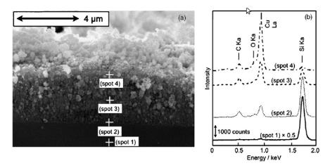
Figure 72: Copper electrodeposition in mesoporous silicon: (a) cross-sectional view of the mesoporous silicon after the copper filling (same process as in figure (71)); (b) EDX spectra analyzed at identified spots in (a). The solid, dotted, dashed and chain lines indicate the EDX spectra at the spots 1, 2, 3 and 4, respectively [35].
