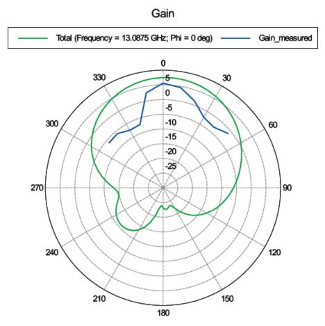
Figure 142: Comparison between measured and simulated radiation pattern.
