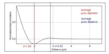
Figure 105: RAA of the macro-PS surface for the buried microporous layer samples.
