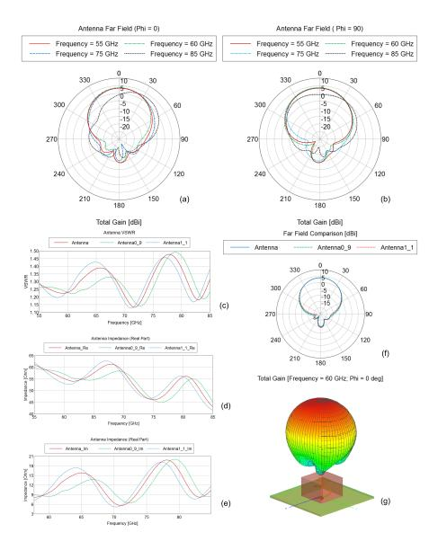
Figure 130: 55 GHz u-helix antenna characteristics for three different heights:  $H_{tot}$ ,  $H_{tot} + 10\%$  (identified by 1\_1), and  $H_{tot} - 10\%$  (identified by 0\_9). Far field gain for the optimized antenna (a, b); VSWR for the three different heights (c); real and imaginary part of the antenna impedance for the three heights (d, e); comparison of the far field gain at 60 GHz for the three heights (f), and solid of radiation of the antenna at 60GHz (g).
