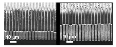
Figure 69: FE-SEM cross-sectional images of macroporous silicon after electrodeposition of Cu in 0.1 M CuSO<sub>4</sub> solution in the dark for: (a) 60, and (b) 120 min [33].
