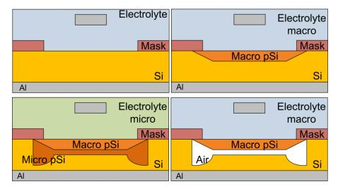
Figure 111: Summary of the technological steps for the realization of buried membranes (left to right, top to bottom).
