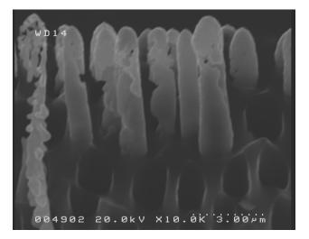
Figure 74: SEM image of the base of the pores obtained in a fractured region of the macro-PS layer.
