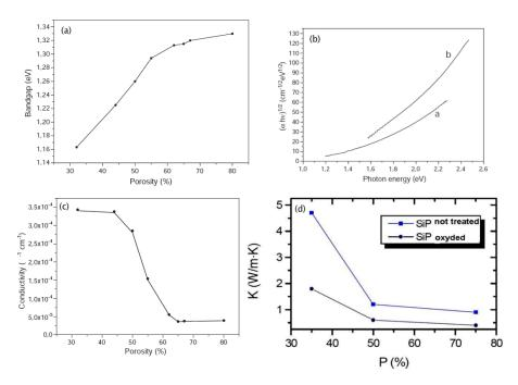
Figure 8: Summary of the properties of meso-PS at different porosities: (a) bandgap [18], (b) absorption [18], (c) electrical conductivity [18], and (d) thermal conductivity for fresh and oxidized (1h in dry O<sub>2</sub>) samples [19].
