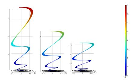
Figure 128: FEM simulation form the 55 GHz u-helix antenna. Deformation and spacing between arms of the metal conductor at three different displacements (from left to right: 3.57 mm, 2.25 mm and 1.6 mm) for a 0.01 mm thick copper metal layer. All dimensions are in mm and the color scale represents the displacement.
