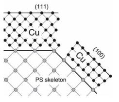
Figure 60: Growth of crystalline copper of different orientation on PS skeleton.
