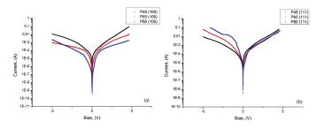
Figure 62: I-V characteristics of Cu/PS structures for (100) (a) and (111) (b) silicon substrates(n-type, 0.01  $\Omega$ *cm*).
