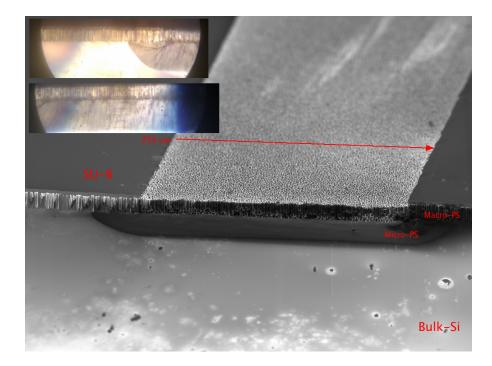
Figure 103: SEM image of micro-PS layer grown below macro-PS. The insets shows optical (50x objective, 7.4  $\mu m$  mark) images of the edge (top inset) and center (bottom inset) of the microporous layer., a) center, b) edge. The sample is realized in HF:DMSO (10:46) with 10  $mA/cm^2$  for 30 min, and HF 45% with 40  $mA/cm^2$  120 min, at RT.
