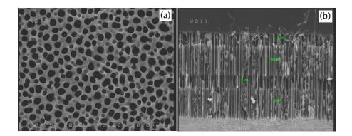
Figure 99: a) SEM image of a multi-layer macroporous silicon structure. The sample has been realized with two steps of organic/aqueous electrolyte alternation: 45 min for HF : DMSO and 5 min for HF : DI : EtOH, for 100 min total process time, at RT.
