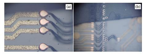
Figure 88: Optical microscope image of pulling pads bonded to the RDL (a); contacting assembly half-filled with a transparent polymer, pyramidal probes are visible in the center (b).
