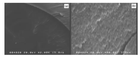
Figure 53: SEM image of micro-PS: edge (a), and its magnification (b). The sample is realized in HF 45% with current density of 40  $mA/cm^2$  for 5 minutes.
