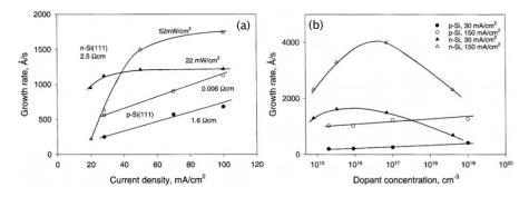
Figure 21: Growth rate of pores as: (a) function of the anodization current density, (b) doping concentration of silicon electrode. [25].
