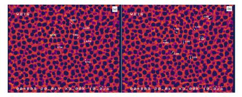
Figure 44: False colors image of the macro-PS layer in figure 42 (b). The diameters of some pores (a) and inter-pores (b) have been high-lighted. All values are in  $\mu m$ .
