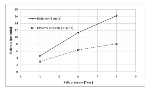
Figure 95: Etch rates for a 1  $cm^2$  surface of silicon. Effective etch rates take into account the purge time between two consecutive etch steps.
