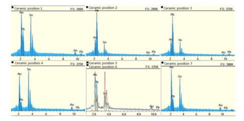
Figure 91: EDX analysis on pad 1(ceramic). Position numbers reflect the one in figure 89. The normalized results are: Pb 29 wt.%, Au 36 wt.% and Sn 35 wt.%.
