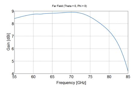
Figure 131: The gain of the 55GHz u-helix antenna in the axial direction in the frequency range of interest. The gain reduction after 76 GHz is due to the tilting of the radiation pattern (see figure 130(a, b)).
