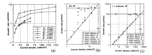
Figure 30: (a) Dependence of pore growth rates on crystal orientations of the substrate for different substrate doping densities and applied current densities (in HF : H<sub>2</sub>O : EtOH, 2:5:1), b) Pore growth rates in (a) 3% aqueous HF and (b) ethanoic HF for different types of substrate doping and doping densities, as indicated. Note that high growth rates are observed for low and moderately doped n-type substrates [17].
