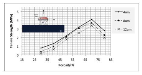
Figure 83: Tensile strength (at break) of porous silicon layers at different porosities for three different metal thicknesses. The measurement setup is shown in the top-left inset.
