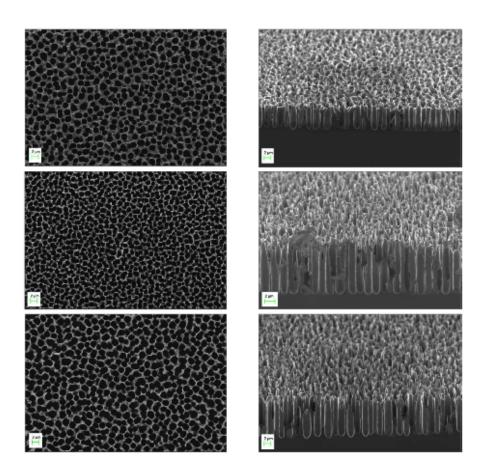
Figure 77: SEM images of macroporous surfaces (top images on left column,  $63^{\circ}$  tilted cross sections on right column) obtained with the processes detailed in table 5: images are ordered from A to C as they appear in the table. The scale on the images corresponds to  $2\mu m$ .
