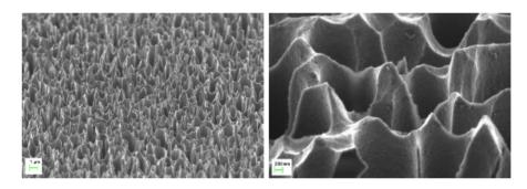
Figure 78: Surface of the sample obtained with B process ( $10 \text{ } mA/cm^2$ , 30 min). Shallow inter-pores are visible as well as the partial dissolution of pore walls.
