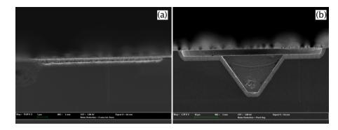
Figure 87: SEM cross sections of low adhesion porous silicon layer (a) below the pyramid region, and high adhesion porous silicon layer (b) below wire region.
