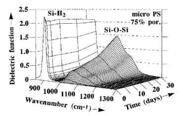
Figure 33: The increase in the Si - O - Si vibrational modes (980-1200 cm<sup>-1</sup>) upon storage of a high porosity (75%) micro-PS layer formed on a p-type substrate (0.2 cm) in ambient air. The Si - H<sub>2</sub> scissors mode (905 cm<sup>-1</sup>) shows little time dependence [29].
