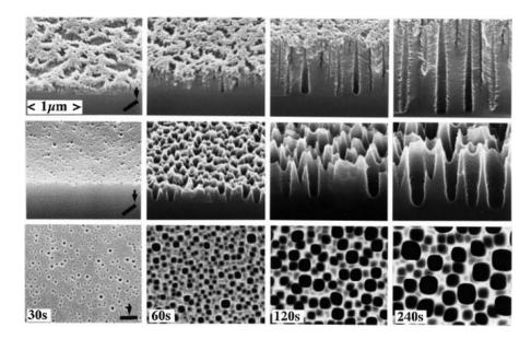
Figure 12: SEM micrographs of surface and cross section of an 0.4  $\Omega cm$  n-type (100) silicon electrode anodized for the indicated times under white light illumination of the front side (2.5% HF, 10 mA cm<sup>-2</sup>, 14 V). Microporous silicon covering the macropores, as shown in the top row, has been removed by alkaline etching for better visibility of the macropore initiation process in the center and bottom rows [21].
