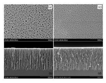
Figure 40: 50% porosity meso-PS layers on n+ type: (100)-oriented silicon wafer (left) and (111)-oriented silicon wafer (right) with resistivity of 0.01  $\Omega$ cm.
