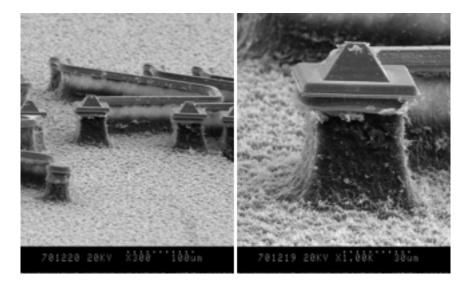
Figure 97: Contact probe (RIE etching testing samples). The wires are all above the polymer in this sample. It is evident the masking effect of the metal wires on the polymer.
