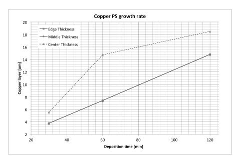
Figure 73: Copper electrodeposition process rate.
