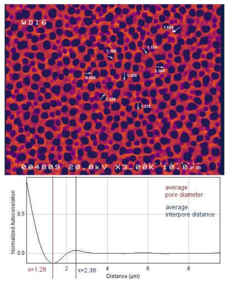
Figure 100: RAA analysis of the multilayer macroporous surface.
