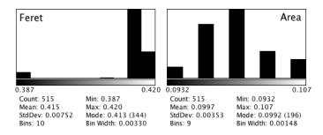
Figure 149: Distribution of the Feret's diameters and holes areas.
