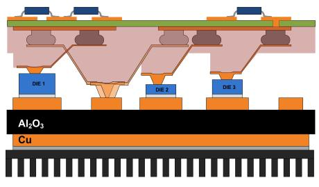
Figure 119: An improved IHPM with the same connectivity exploiting the top board to replace two long wires contacting the substrate.
