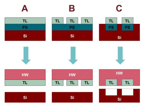
Figure 81: Three different layer transfer technologies employing porous silicon as sacrificial layer.
