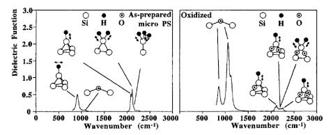
Figure 32: Characteristic dielectric functions (imaginary part), as observed by IR spectroscopy for the solid component of as-prepared PS (left) and an oxidized sample (right), with the most important vibrational modes assigned as indicated [17].
