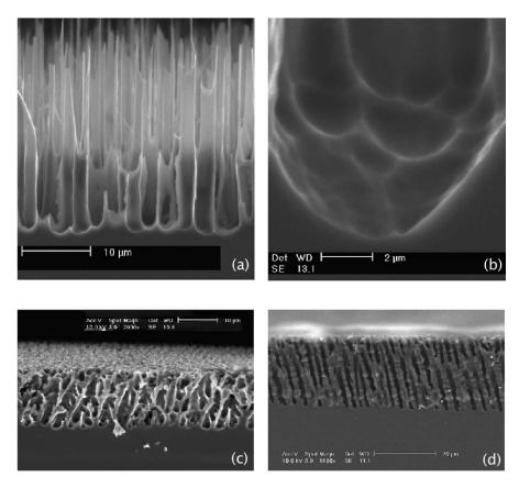
Figure 27: Some samples of macro-PS produced with aqueous solutions: (a) 10  $\Omega cm$ ; 7% *HF*, j = 20  $mA/cm^2$ ,  $j_{PSL}$  = 90  $mA/cm^2$ , random nucleation; (b) as (a), but induced nucleation (hexagonal lattice, a = 3 *mm*); (c) 10  $\Omega cm$ ; 10% HF, j = 2  $mA/cm^2$ ,  $j_{PSL}$  = 150  $mA/cm^2$ , random nucleation on (5, 5, 12) sample; (d) p-type silicon produced with organic solutions with MeCN (4 wt.% HF) on (111) for comparison with (c)[27].
