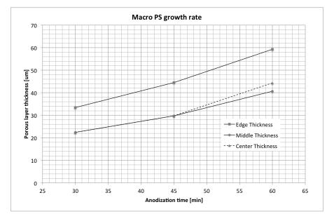
Figure 51: Macro-PS growth for HF:DMSO (10:46) on p-type (100)-oriented, 10-20  $\Omega cm$  silicon wafer. Data are sampled in three different points (see 3.3.3 for a description of the sampling strategy).
