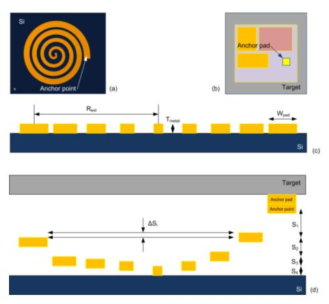
Figure 136: On-chip integration of u-helix antennas. The substrate hosting the antenna is bonded to an I/O pad of the RF IC using a suitable interconnection technique: copper pillar, gold-to-gold bonding, etc.
