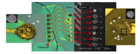
Figure 89: Detail of a gold finished sample (silicon left, ceramic right) after pulling process. Pad 1 (both sides) is magnified to show micro and quantitative analyses areas. The visible film on optical photo (left) is a residue of flux used for solder reflow. The probing tips (at the left) are still attached to the surface even if corresponding wires have been completely released.
