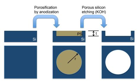
Figure 4: Gravimetric method for evaluation PS porosity. The weight of a silicon sample (cross-section and top-view) is measured before and after anodization (the porosification process) and a third time after the removal of the porous layer, e.g. by immersion in a KOH solution.
