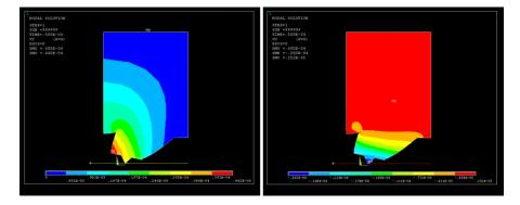
Figure 98: FEM simulation of the electrical contacts realized with the CRML technology. The vertical (left) and lateral (right) displacement fields are shown.
