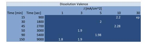
Figure 47: Dissolution valence for the macro-PS samples realized in the experiments reported in table 4. Electropolishing (ep) is reported for  $30 \text{ } mA/cm^2$ .
