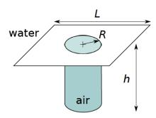
Figure 79: Idealized lattice used to model the macro-PS surface used for calculation. Air is trapped inside the cylindrical pore of radius R and height h. Water is in contact with the whole (periodic) cell of lattice constant L and area  $L^2$ .
