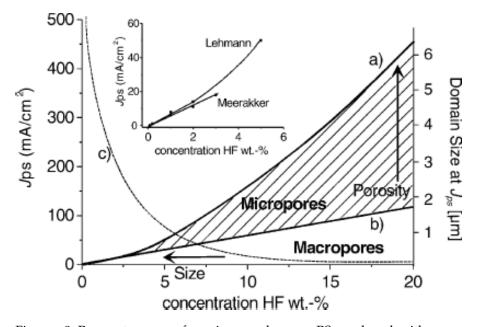
Figure 28: Parameter space for micro- and macro-PS produced with aqueous solutions. Curve (a) shows  $j_{PSL}$  as described by the Lehmann [26] model and curve (b) as described by van den Meerakker [28]. Curve (c) describes the size of a CB domain. The regions for macropore and micropore-growth are a result of a semi quantitative consideration of the CBM and may be considered as a prediction. The inset shows measured data taken from [28, 26] for low HF concentrations [27].
