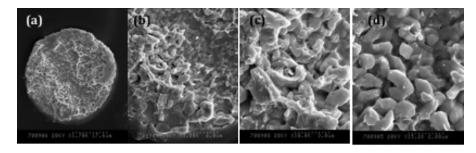
Figure 93: SEM analysis of pad 5 on ceramic substrate: (a) full pad view, (b) particular of the bottom left area, (c) and (d) intermetallics.
