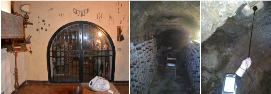
Figure 4: Some photos of the cellar in the basement. Left: the wrought-iron door communicating with the living room. Centre: the cellar, dug in peperino and ground (the AlphaGuard is lying on a chair). Right: the venting hole in the cellar ceiling, during an air-flow measurement.
