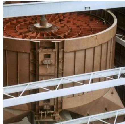
Fig. 2. Rotating matrix of a Ljungstrom heat exchanger
