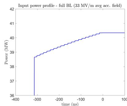
Figure 3: Input RF pulse for ideal beam loading compensation. The first bunch has to be injected at t=0.
