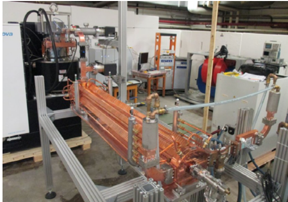
Figure 6: High-Order Mode damped C-band accelerating RF cavities, designed and built by INFN-LNF for EuroGammaS, under full power test.
