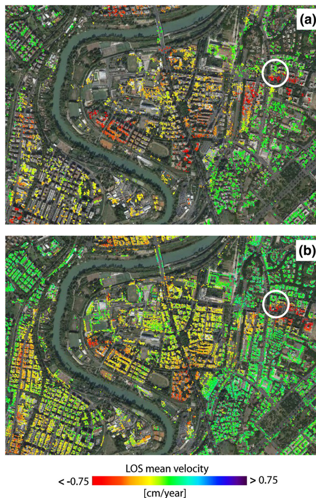
Fig. 3 Comparison between the ERS/ENVISAT and CSK SBAS-DInSAR results relevant to the selected area identified by the black box in Fig. 2. a Zoomed view of the full-resolution SBAS-DInSAR results achieved through the 1992–2010 ERS/ENVISAT SAR data archive for the investigated area. b Zoomed view of the full-resolution SBAS-DInSAR results achieved through the 2010–2012 CSK SAR data archive for the selected area. The white circles indicate the position of the investigated building
