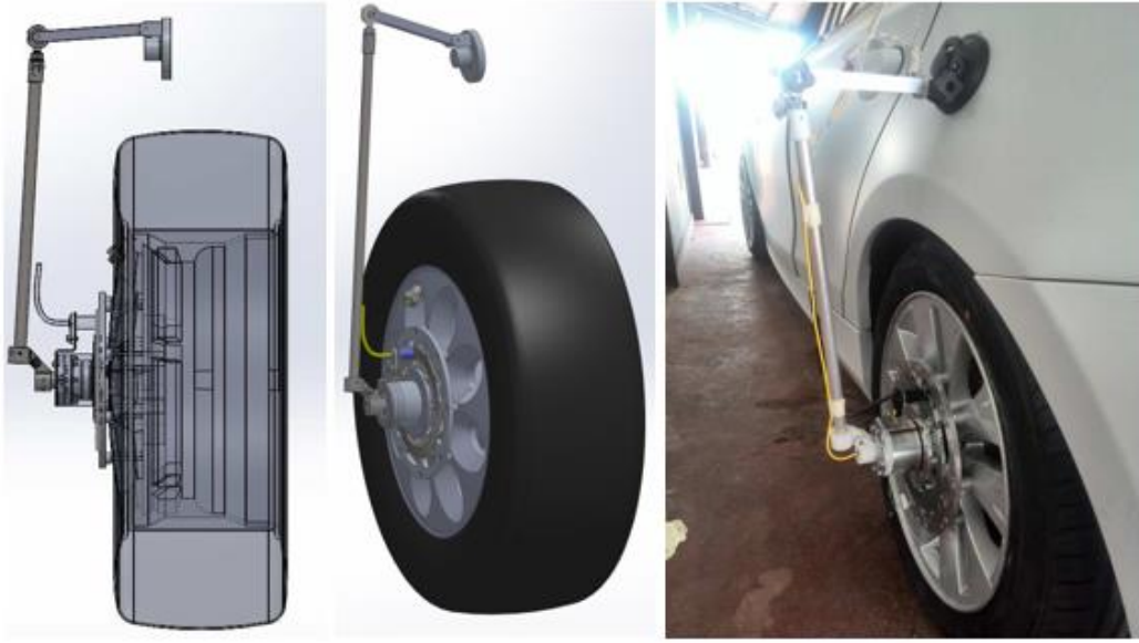
Figure 4: Support case onboard installation.
