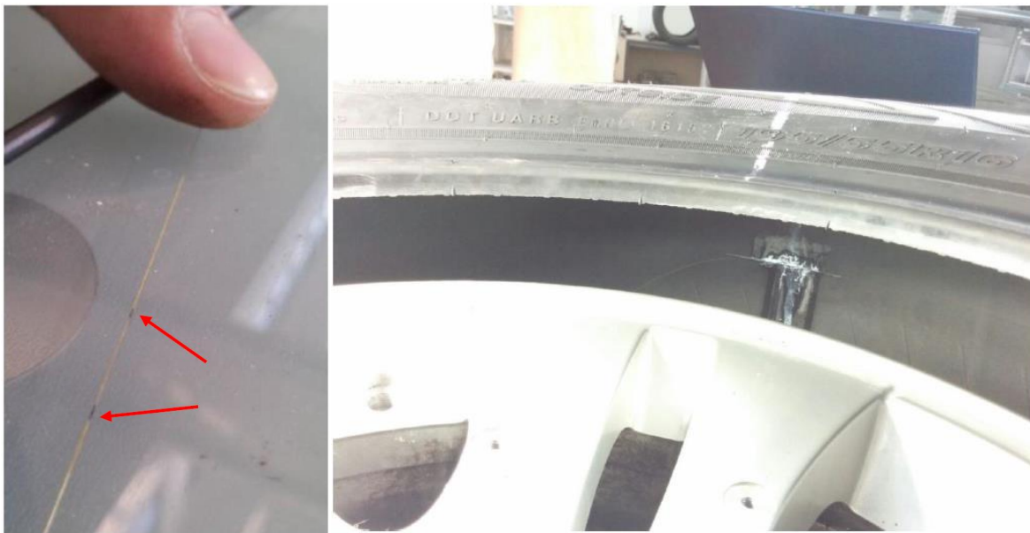
Figure 1: On the left, the optical fibre with one FBG, the sensor lies within the black marks on the line, on the right, the optical fiber pasted into the inner liner of the tire.
