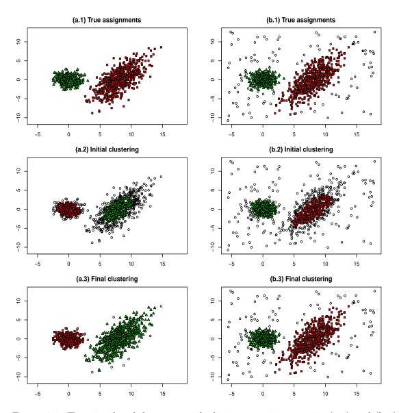
Figure 3.1: Two simulated data sets with their true assignments in (a.1) and (b.1). The result of TCLUST with  $\alpha_0 = 0.33$  in (a.2) and (b.2). The final assignments obtained after applying the proposed methodology are given in (a.3) and (b.3). Noisy data and trimmed are denoted by  $\circ$  in all graphs throughout the manuscript.
