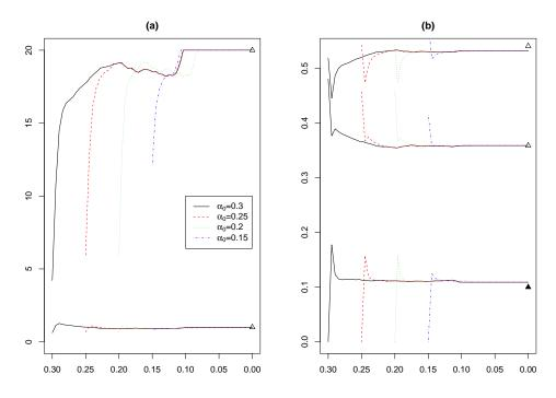
Figure 3.2: Evolution of  $|\Sigma_j^l|$  in (a) and of  $\pi_j^l$  in (b) for different initial  $\alpha_0$  values  $(\alpha_0 = .3, .25, .2 \text{ and } .15)$  for the data set shown in Figure 3.1 (b.1). The up-triangle symbols are the true parameters to be estimated.
