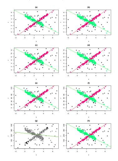
Figure 4.3: Different degrees of fuzzification obtained for different scale values s ( $y_i$  is replaced by  $y_i \cdot s$ ). m = 1.5 and s = 0.5 in (a); s = 1 in (c); s = 10 in (e); s = 32 in (g). m = 1 (hard clustering) and s = 0.5 in (b); s = 1 in (d); s = 10 in (f); s = 32 in (h).
