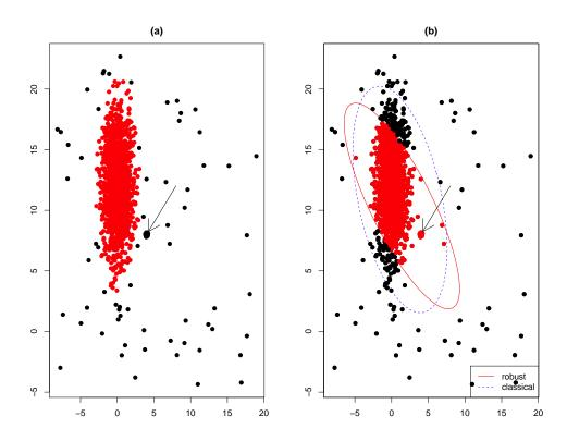
Figure 3.4: (a) The proposed iterative reweighting procedure when k = 1 started from  $\alpha_0 = 0$  and  $\alpha_L = 0.01$  (b) The (traditional) reweighted MCD started from  $\alpha_0 = 0$  and  $\alpha_L = 0.01$ . Trimmed points are the black points.
