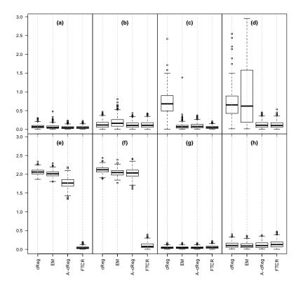
Figure 4.9: Simulation study. Boxplots representing the MSE of  $b_j$  and  $b_j^0$  for setting S1: p = 1, k = 2. The Homoscedastic clusters are in (a),(c),(e),(g). Heteroscedastic clusters are in (b), (d), (f), (h). Uniform contamination is in (a) and (b). Inflated uniform contamination is in (c), and(d). Pointwise contamination in (e) and (f). Clean dataset is in (g) and (h)
