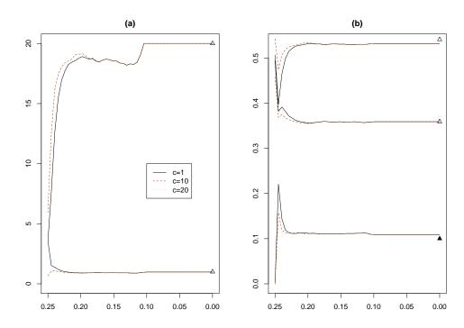
Figure 3.3: Evolution of  $|\Sigma_j^l|$  in (a) and of  $\pi_j^l$  in (b) for different initial c values (c = 1, 10 and 20 while the true c needed was 11.71) for the data set shown in Figure 3.1 (b.1). The up-triangle symbols are the true parameters to be estimated.
