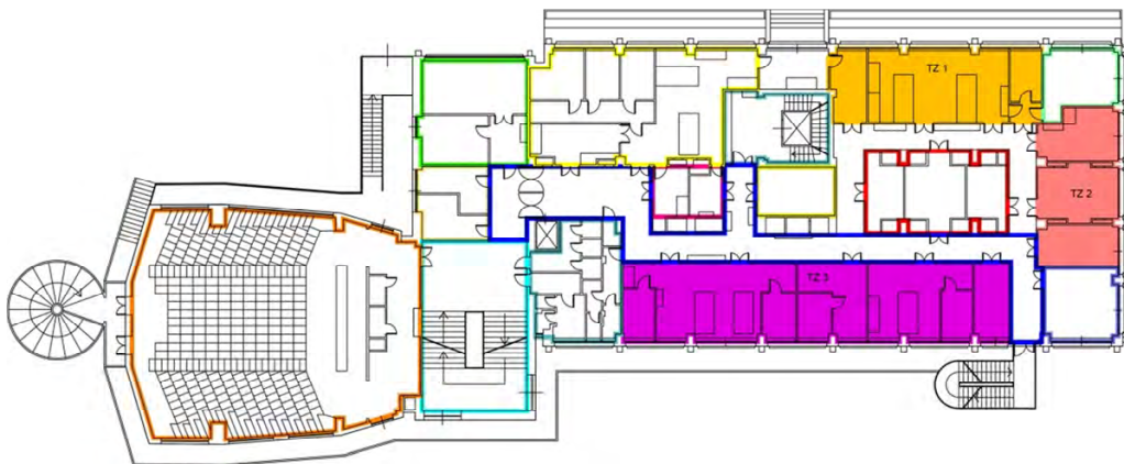
Fig. 2. Thermal zones division of the second floor.
