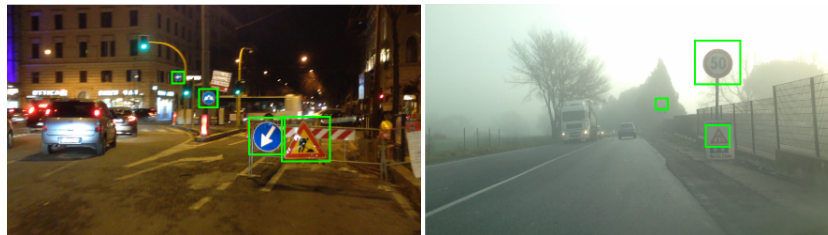
Fig. 5. Two annotated images from the DITS data set captured at night time (left) and with fog conditions (right). Annotations are shown in green.
