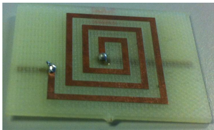
Figure 3-8: showing the fabricated inductor and the solder spheres created at each end of the coil
