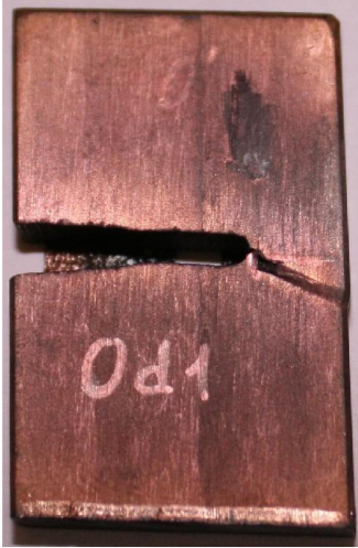
Figure 3.13: Specimen r-UD_0d1 (picture): macroscopic kink band.
