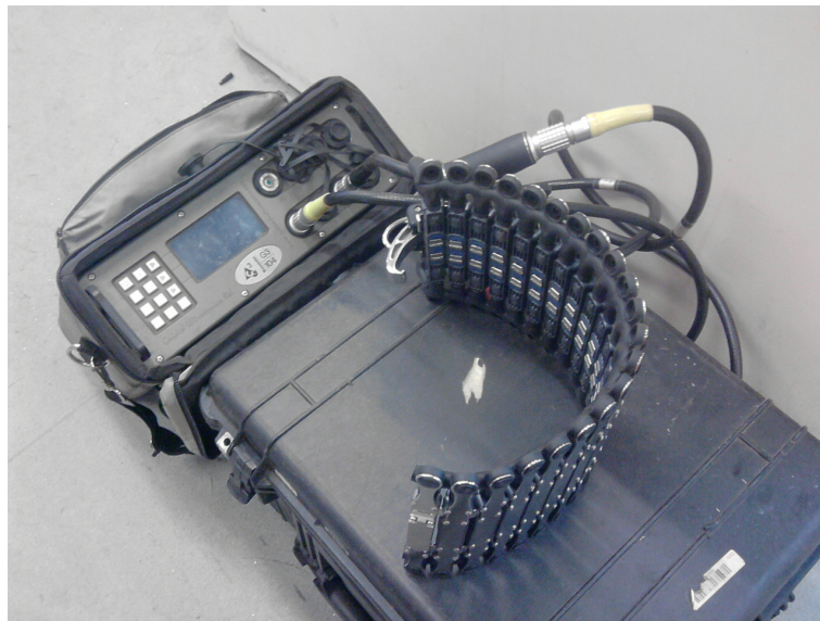
Figure 2.11: Picture of commercial guided wave equipment produced by Guided Ultrasonics Ltd. This is the G3 instrument attached to a low-profile 5 inch solid transducer ring.
