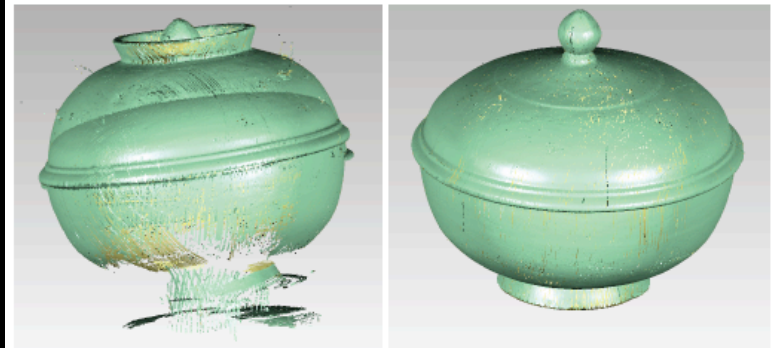
Fig. 4. Left, the two views of the same object do not naturally fit together after scanning. On the right, after cleaning the multiple views, 3D registration is performed aligning the two parts of the model together.
