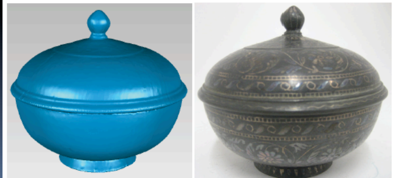
Fig. 5. After 3D registration the point clouds of the two scans are fused into a single object and transformed into a triangulated surface shown on the left blue model. On the right, texture mapping can then be applied to the triangulated surface.
