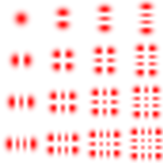
Figure 1.2: Intensity distribution of the first 20 Hermite-Gaussian modes in a laser cavity with rectangular symmetry calculated according to [22].
