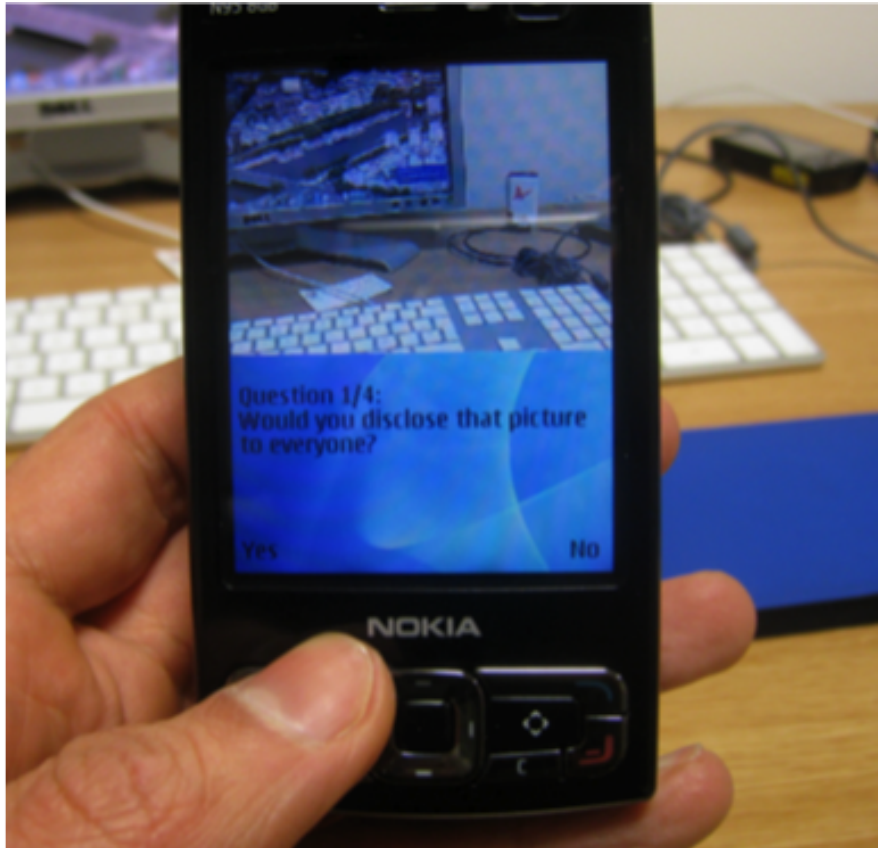
Fig. 3 The LocShare application running on a Nokia N95 smartphone as used in our experimental testbed. The participant is asked whether he/she would share a photograph with his/her social network friends.
