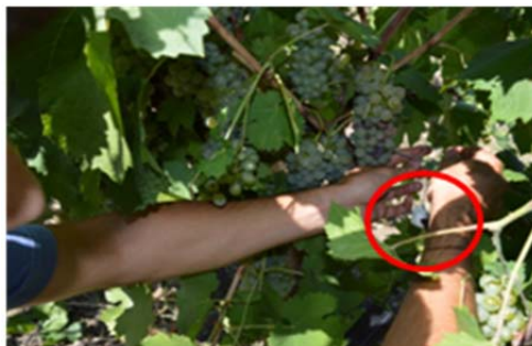
Figure 2: The non-commercial instrumented sphere used in the tests while positioned on the first wire of the hedgerow.
