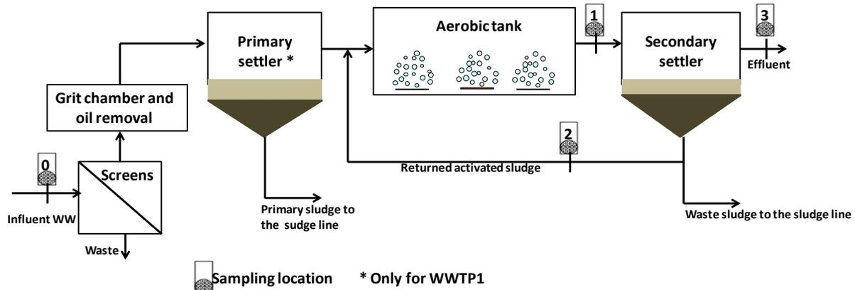
Figure 1. Lay out of each investigated WWTP
