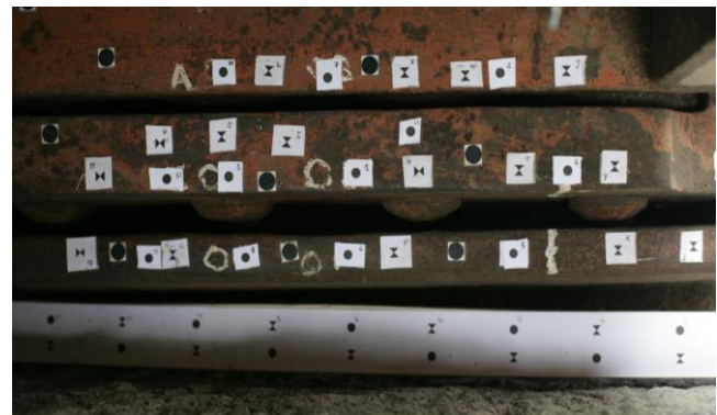
Figure 10. Frame with control points and tie points disposed on the support device
