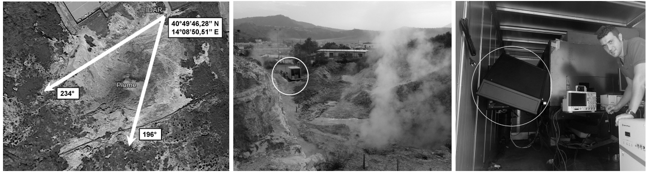
Figure 1. Left) Location of lidar and plume, and most northern/southern directions of the laser beam during the measurements. Center) Volcanic plume emitted by the Pozzuoli Solfatarata in Contrada Pisciarelli. The lidar is mounted in a small truck (inside the white circle). Right) Lidar inside the truck. The laser beam is aimed by two large elliptical mirrors (major axis: 450 mm) mounted in two black boxes (inside the white circle).
