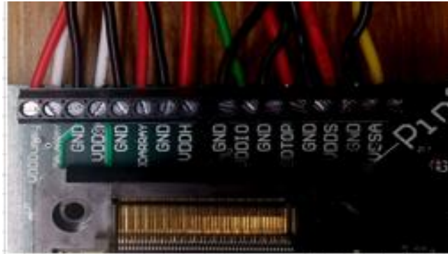
Figure 2-21 Power connections on the custom PCB
