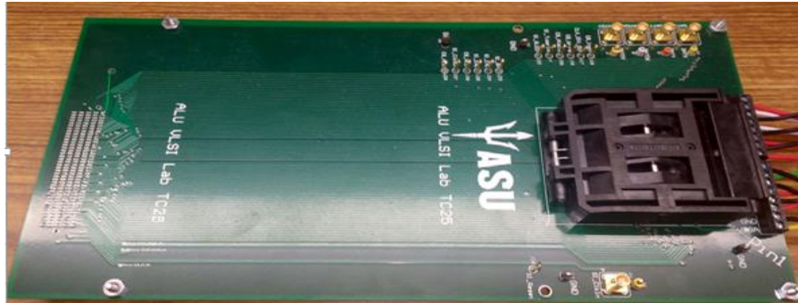
Figure 2-3 Custom PCB of TC25 post silicon validation setup
