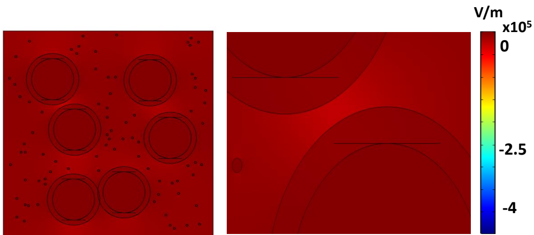
Figure 43: Electric field distribution in the specimen with debonding represented as an elliptical area
