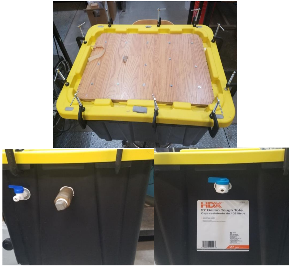
Figure 4: Carbonation tank developed for iron carbonate binder synthesis
