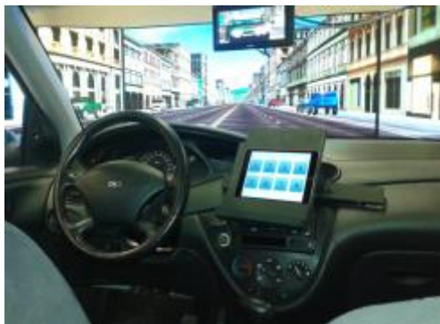
Figure 22. Driver's View of the Simulator with 10" Tablet
