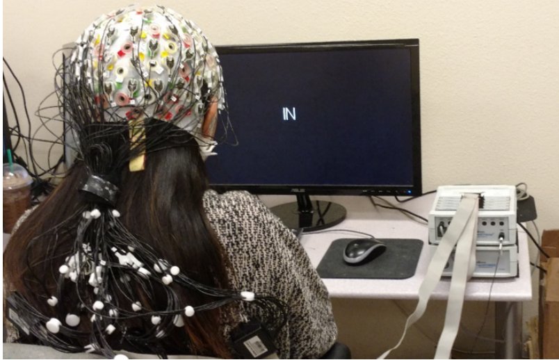
Figure 5.1: Experimental setup. The subject is wearing the cap with EEG electrodes and looks at a monitor a few inches away. The monitor shows the task that the subject must execute. In this illustrative figure, the subject was imagining pronouncing the word “in”.
