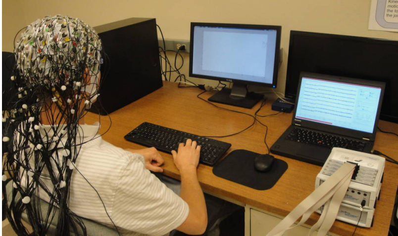
Figure 3.1: Subject in front of the monitor wearing the EEG cap and electrodes. (Karavas and Artemiadis (2015), ©2015 IEEE)
