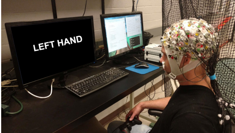
Figure 4.1: The subject is wearing the cap with EEG electrodes and looks at a monitor a few inches away. The monitor shows the task that the subject must execute. In this case the subject must imagine moving his left hand. (Karavas et al. (2017), ©2017 IEEE)
