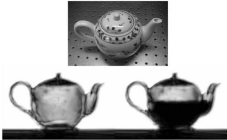
FIGURE 2.4: The image of a teapot by using Gunn diode and a Schottky diode detector at 200 GHz. The upper image is the photograph for the teapot. The image on the left bottom is the THz image without water inside and the one on the right is with the water inside (cited from Hu, Q, 2008).
