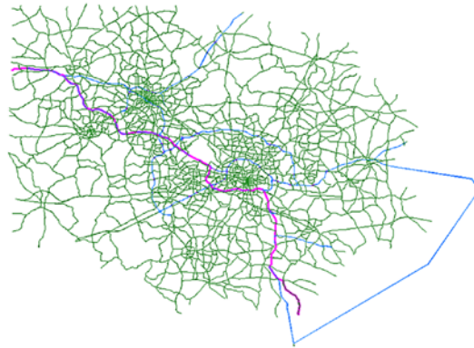
Figure 16. Triangle Regional Model, NC network with 2,389 zones, 20,259 links, about 2,000 signalized intersections, 1.06 million vehicles in morning peak hours.
