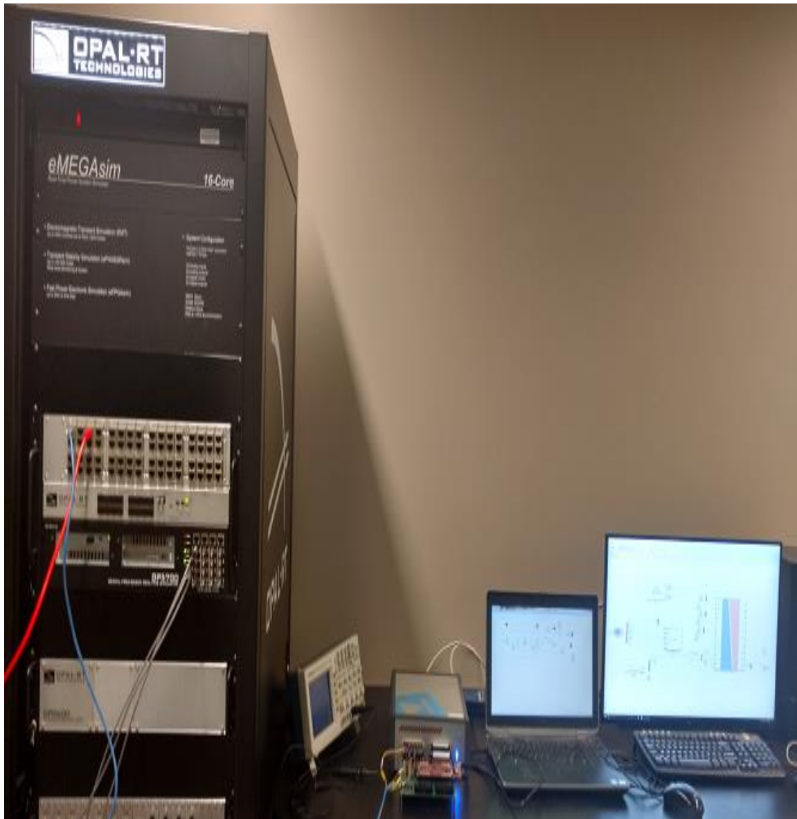
Figure 4.9 – PLECS –RT box model integrated with the OPAL-RT model
