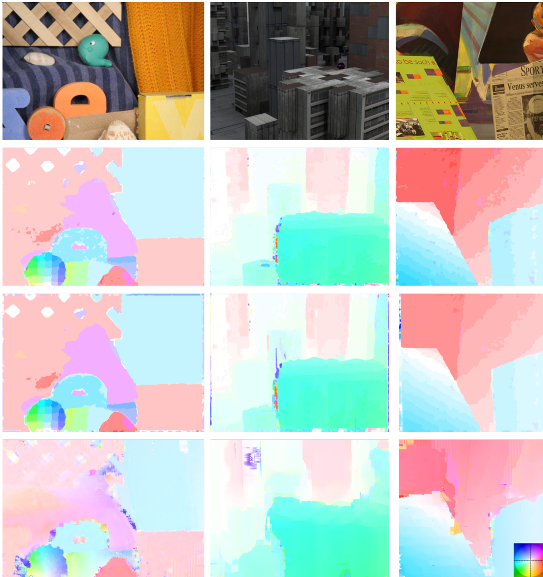
Figure 5.2 Colored flow maps for 3 types of scenes using different algorithms. 1 st column: RubberWhale; 2 nd column: Urban2; 3 rd column: Venus. 1 st row: input previous frame; 2 nd row: NG-fSGM; 3 rd row: fSGM; 4 th row: Lucas-Kanade. Color legend is at bottom-left corner.
