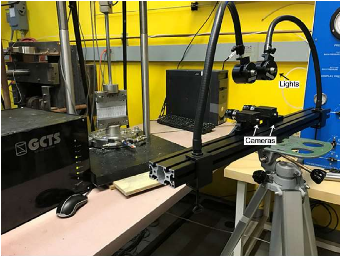
Figure 6-6: DIC image capture equipment setup
