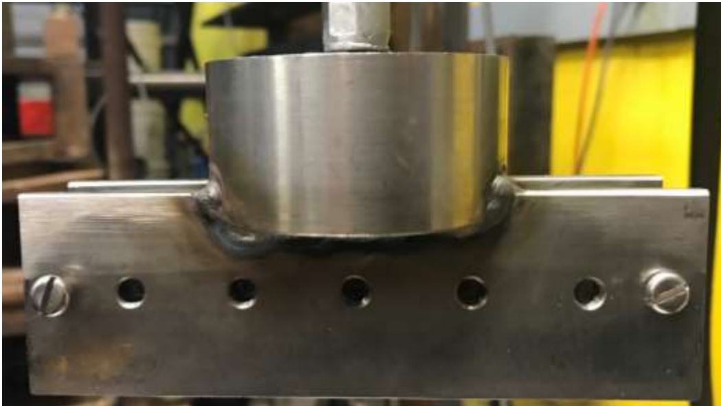
Figure 6-4: Upper grip apparatus (front view)
