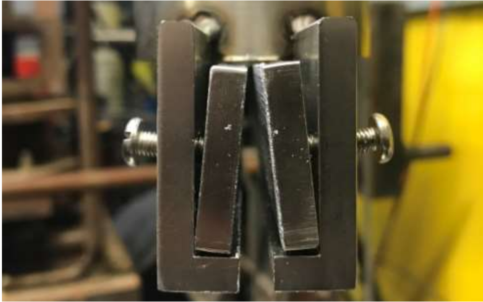
Figure 6-5: Upper grip apparatus with textured load plates (side view)
