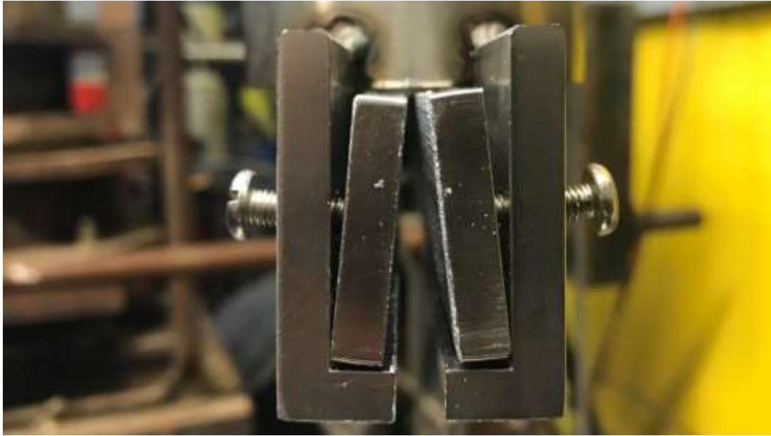
Figure 5-2: Upper grip apparatus with textured load plates (side view)
