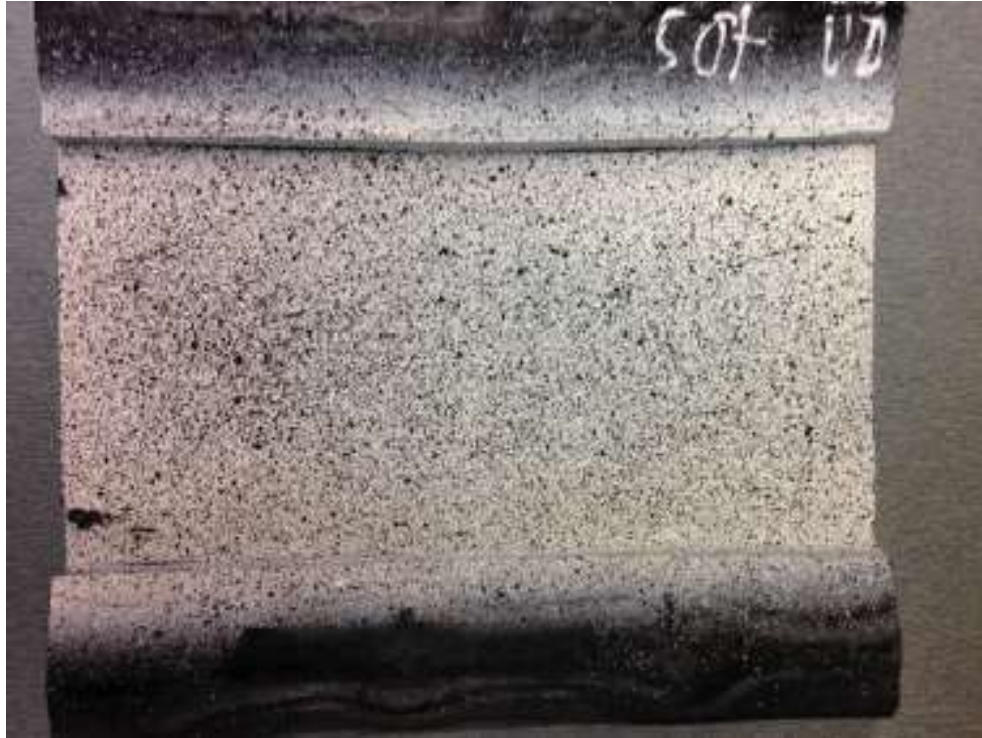
Figure 4-8: HDPE sample prepared with speckle pattern for DIC analysis
