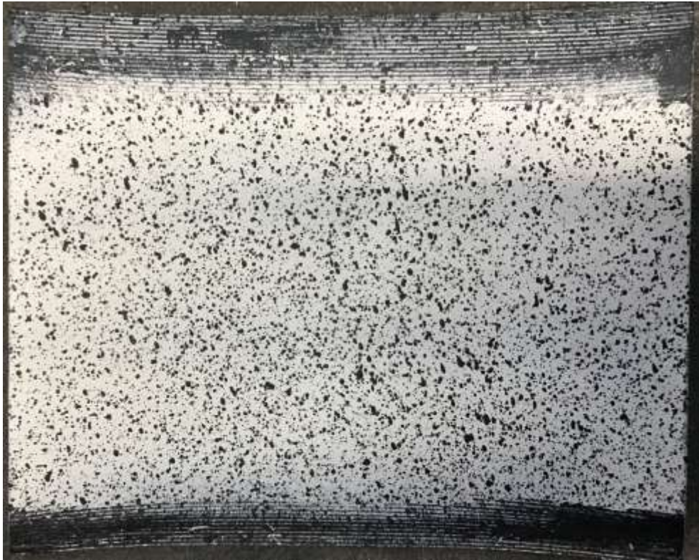
Figure 6-8: HDPE sample prepared with speckle pattern for DIC analysis
