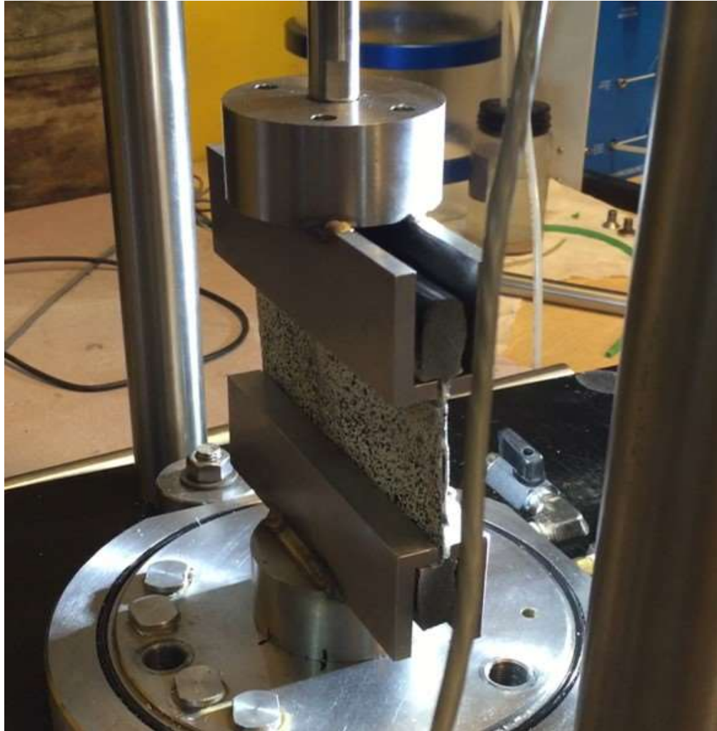
Figure 4-5: Geomembrane clamping and loading system with sample inserted, ready to be tested
