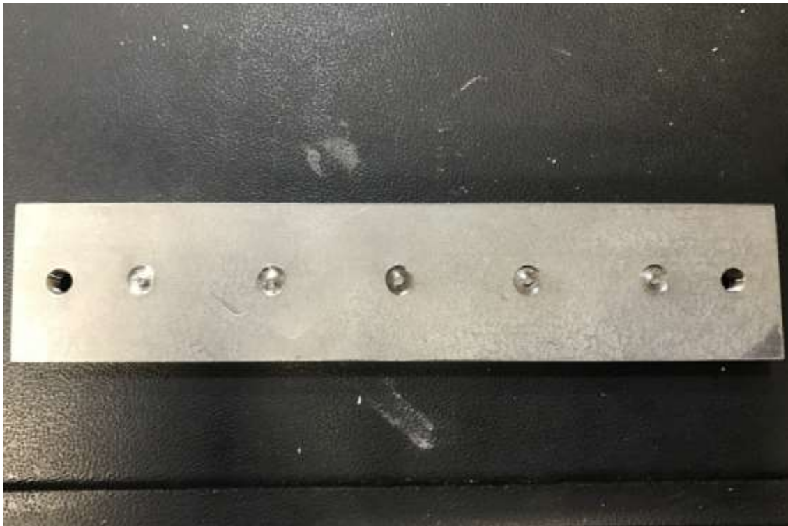
Figure 5-3: Friction plate with dimensions 150 mm wide by 30 mm tall
