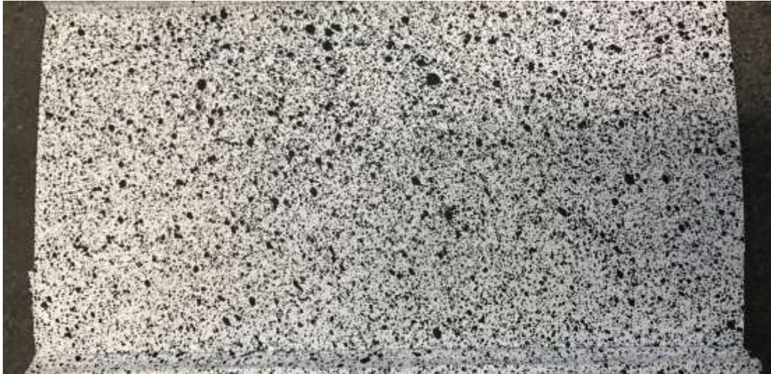
Figure 3-3: Appropriate speckle pattern applied to the surface of an HDPE geomembrane sample
