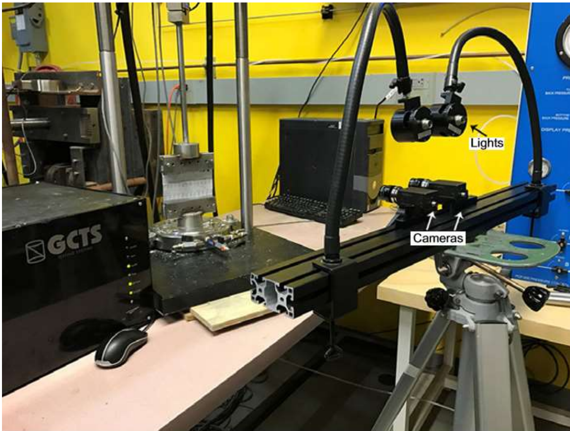
Figure 5-4: DIC image capture equipment setup
