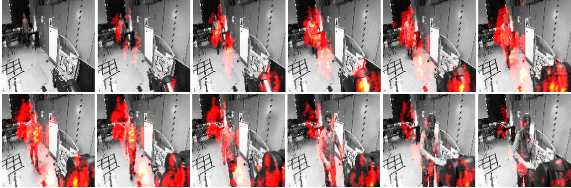
Figure 4.8: Saliency map visualization of p_{t+5} predictor. It anticipates any interactions into the future. The images show, highlighted in red, the pixels the network is paying attention when generating an output. In the beginning, almost no region is active, but as the human starts approaching the robot, the network focuses on the human and also on the robot arm. Once the subject is in contact with the robot, the activations attenuate.
