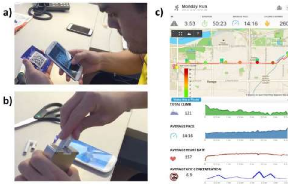
Figure 4.4 (a) Scanning sensor QR code; (b) Replacement of new sensor cartridge; (c) Real-time fitness and VOCs exposure device data during personal exercise.
