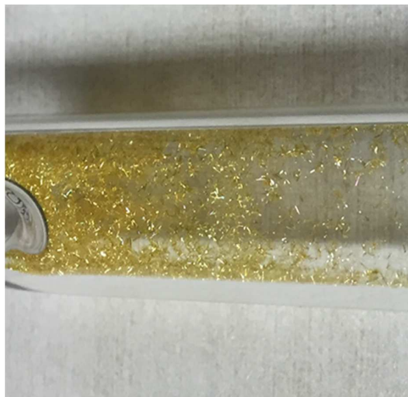
Figure 5. \text{HfS}_3 crystals grown on the inner walls of a quartz ampoule.
