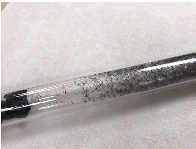
Figure 4. \text{TiS}_3 crystals grown on the inner walls of a quartz ampoule.
