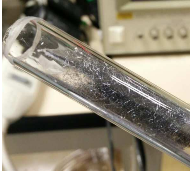
Figure 23. Nb 0.5 Ti 0.5 S 3 crystals grown on the inner walls of a quartz ampoule.
