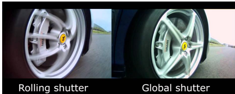
Figure 6 Image of fast moving object with rolling and global readout[13]
