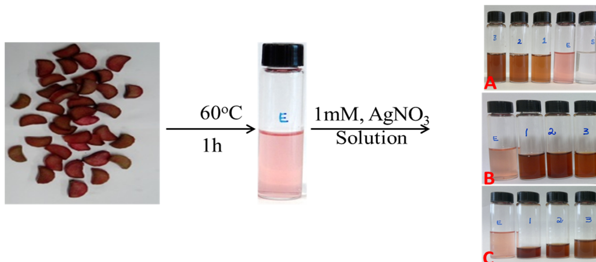
Figure 1 Scheme of GR-SNPs synthesis in different reaction mixture: (A) GR Extract + \text{AgNO}_3 solution variation, (B) both GR extract and \text{AgNO}_3 solution variation and (C) GR extract variation+ \text{AgNO}_3 solution
