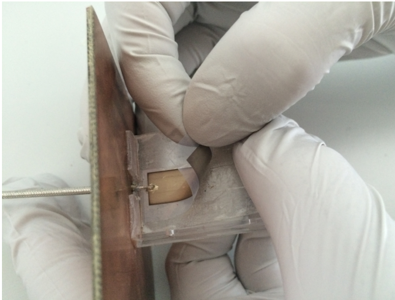
Fig. 5. Demonstration of flexibility of inkjet printed antenna.
