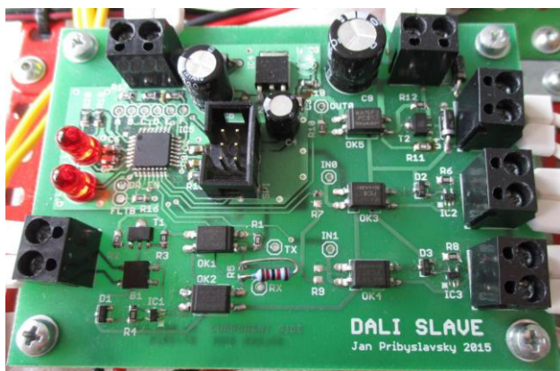
Figure 4. The ready to use DALI Slave I/O unit photo [3].
